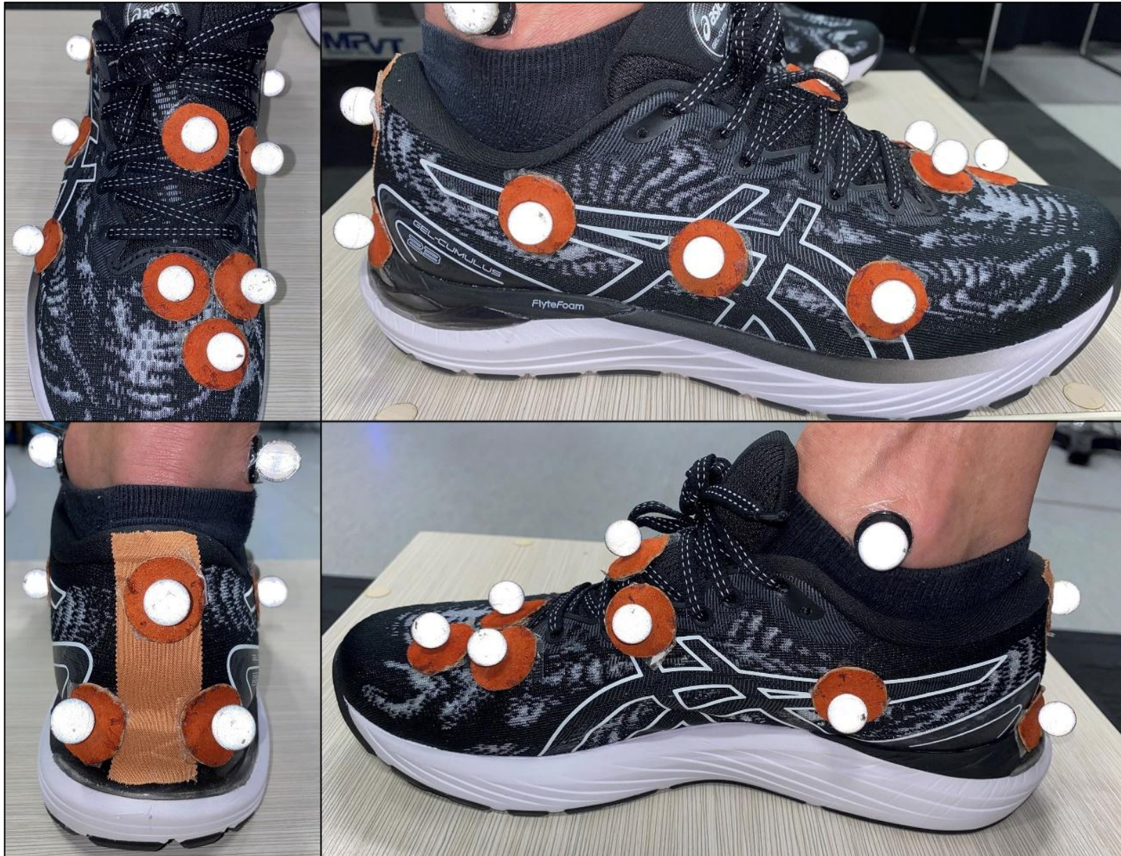
Figure 6.3: Marker placement on the shoe as per the model detailed by Weir et al. (231).
