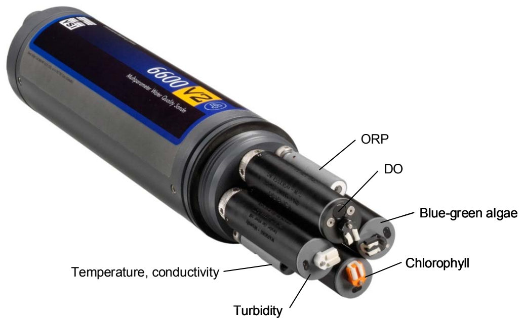
Figure 4. Photograph showing a YSI 6600V2 multiparameter sonde with four self-cleaning optical sensors (wiper) capable of measuring dissolved oxygen, turbidity, chlorophyll and blue-green algae. This sonde also records temperature, conductivity (salinity), pressure (depth), pH, and oxidation–reduction potential (ORP).
