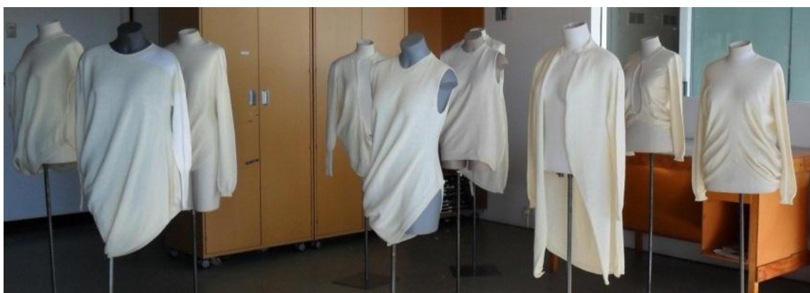
Figure 56: Smith, A. (2011). Seamless garment developments created using 'knitpaint' shapes and one or two additional pacs
