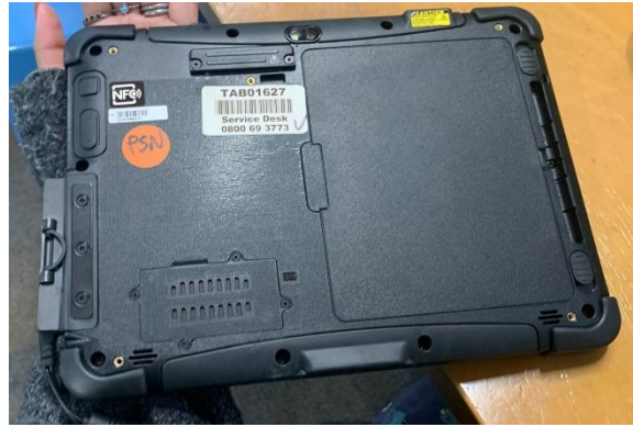
Figure 7: Back of the MDT. There is no communication or camera function on the device itself
