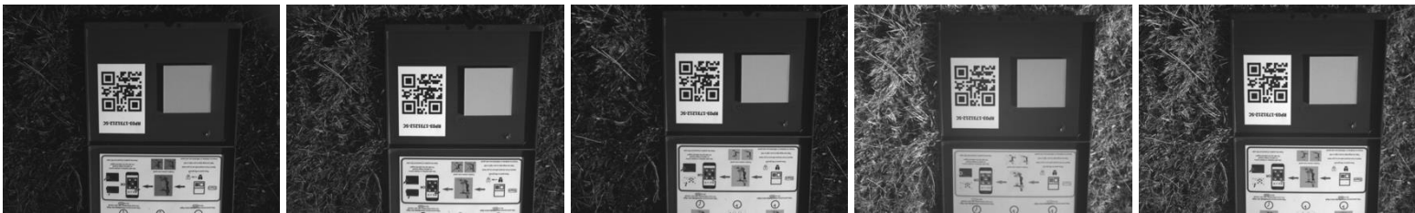
Figure 17: Radiometric calibration panels from Left (Red, Blue, Green, NIR, RED) taken with MicaSense RedEdge Sensor.
