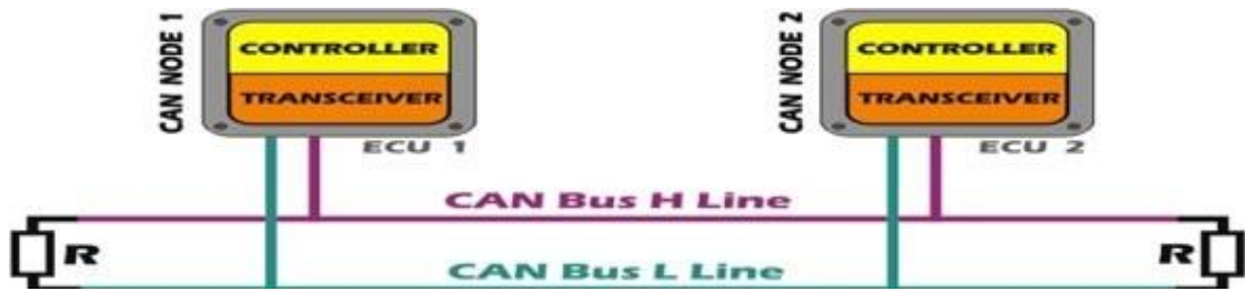
Figure 2.5: CAN Bus Components (CSS Electronics, 2018)
