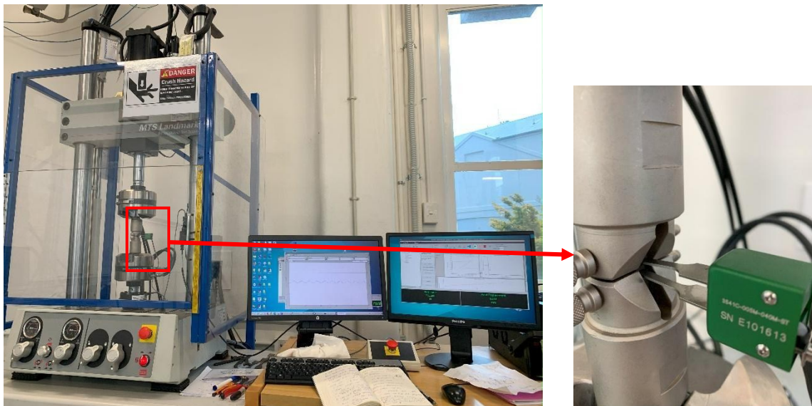
Figure 3.14. Epsilon COD gage used for FCG tests.
