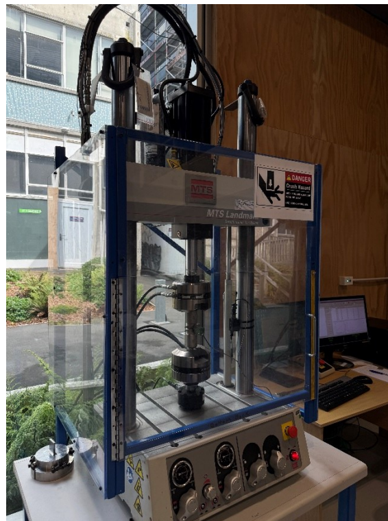
Figure 3.10. Landmark® Servohydraulic Test Systems.
