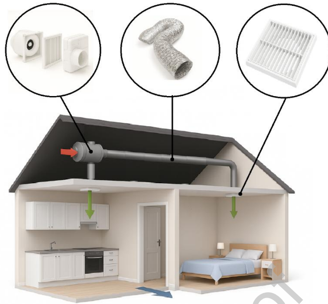
Figure 3 - Typical schematic of PPV home installation, showing details of (L-R) fan/filter assembly, ducting, and diffuser.
