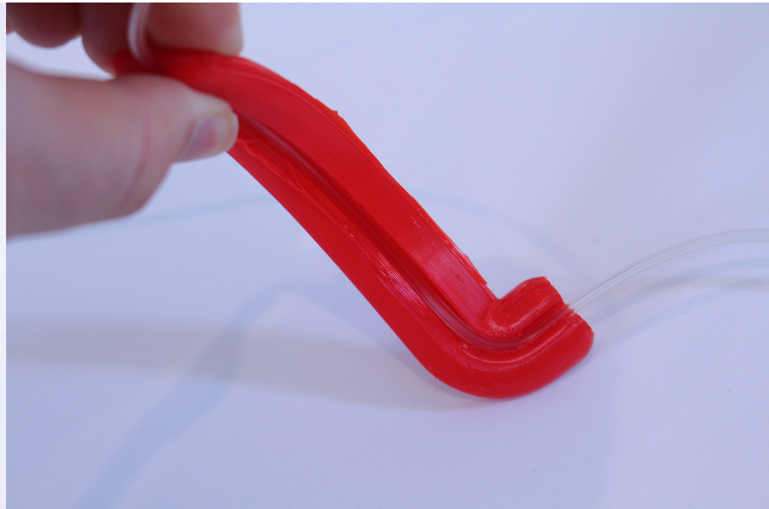
Figure 125. Follow the testing of rigid prototypes, I explored prototypes made from more flexible materials. Two versions were printed with different forms to explore how these would affect flex in the system. Based on these explorations, I found that using a flexible material allowed for a better fit on the patient's skin; however, this was at the sacrifice of a secure fit on the IV line.
