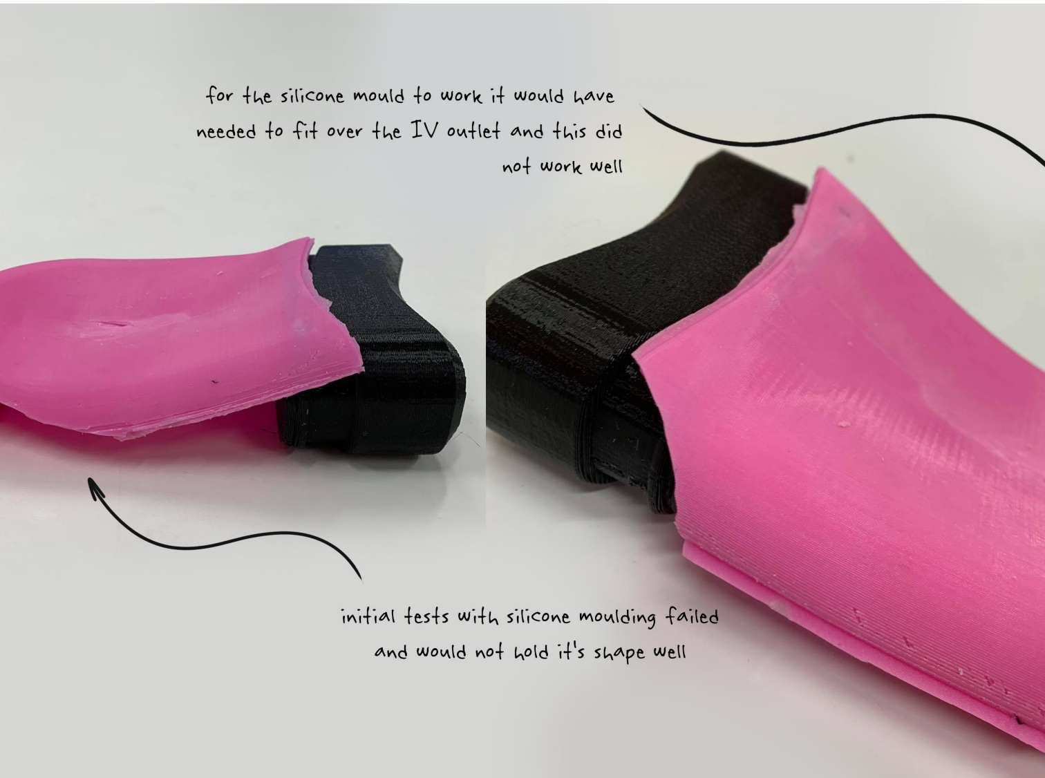
Silicone moulding was tested for the soft-shell infuser; however, getting the silicone robust enough without glue became too complex to be viable quickly.
