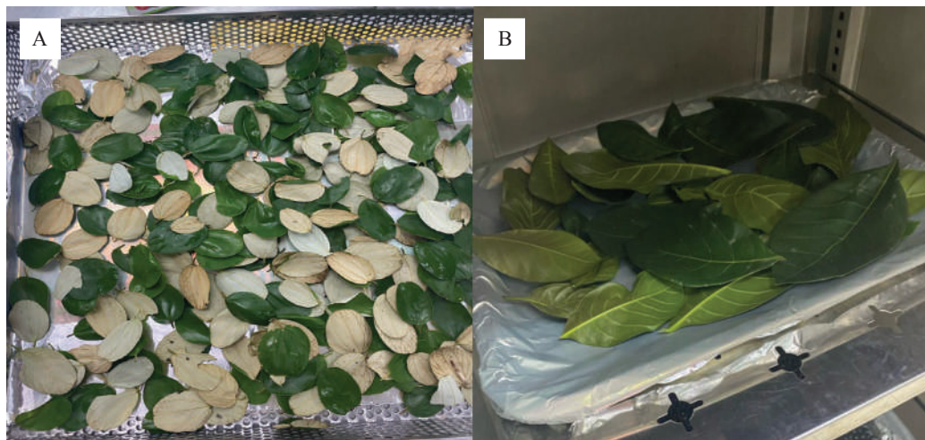
Figure 1: (A) Ziziphus mauritiana and (B) Artocarpus heterophyllus Lam. leaves were subjected to a drying process using a cabinet dryer for 12 hours at 52°C
