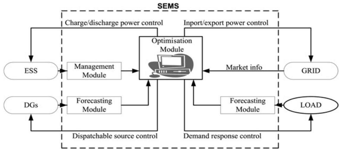
Figure 2.4: Typical illustration of SEMS inputs and outputs
