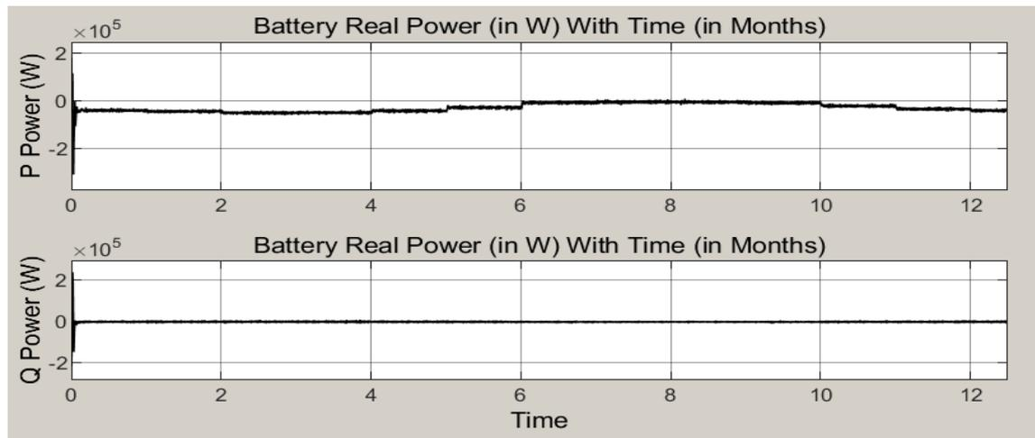
Figure 4.12: Battery operation at saturation's upper and lower limits of 300000 and -300000 respectively
