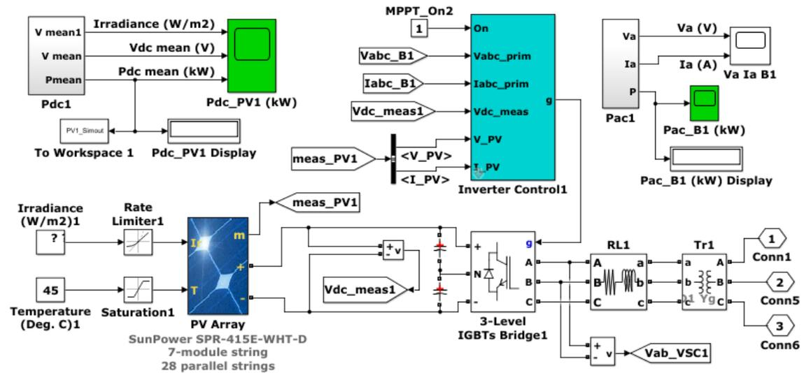
Figure 3.10: Schematics of the inverter control modelled into the design
