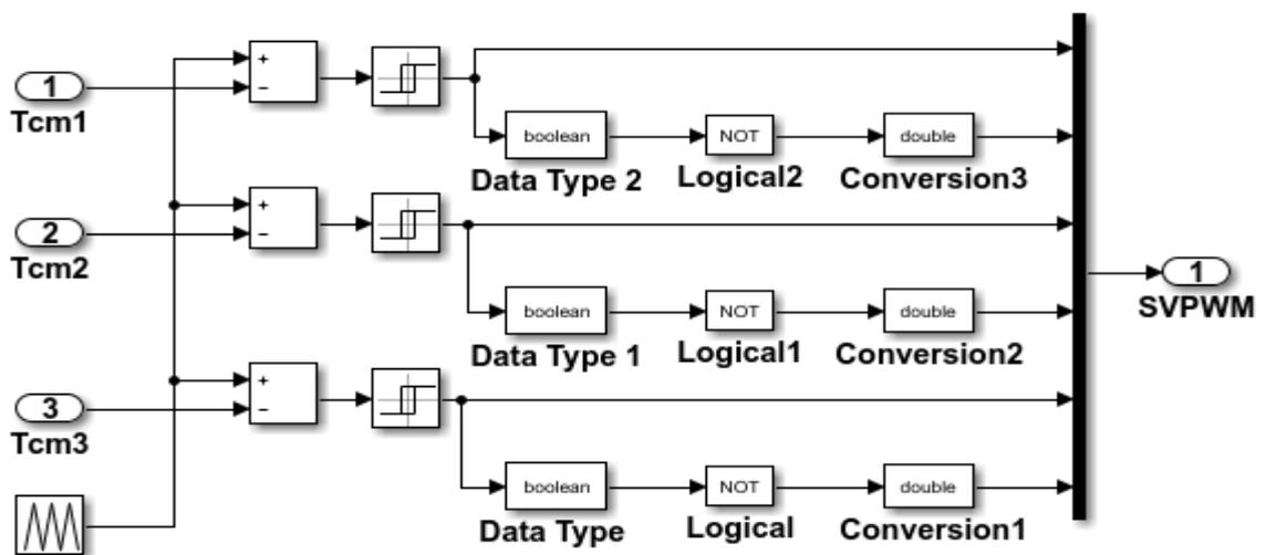
Figure 3.6: Schematics of the Pulse Width Modulation (PWM)
