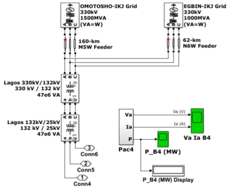
Figure 3.2: Schematics of the two generation plants modelled inside the utility grid subsystem
