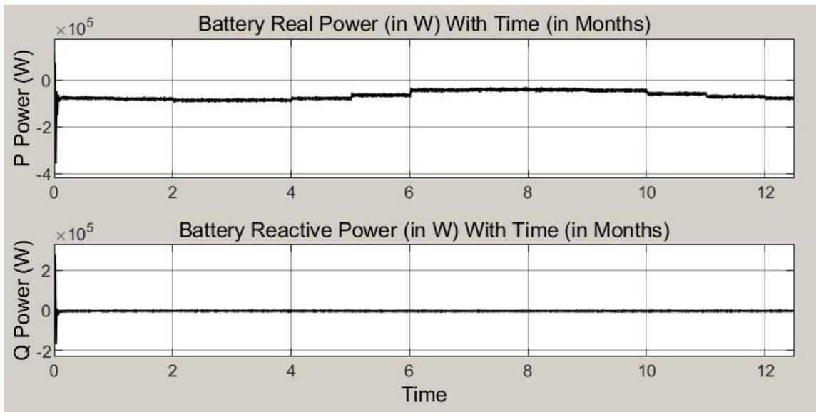
Figure 4.4: Battery operations at upper and lower limits saturation of 300000 and -300000 respectively
