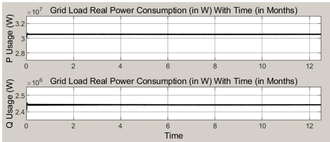
Figure 4.14: Analysis of the 30MW grid load energy consumption
