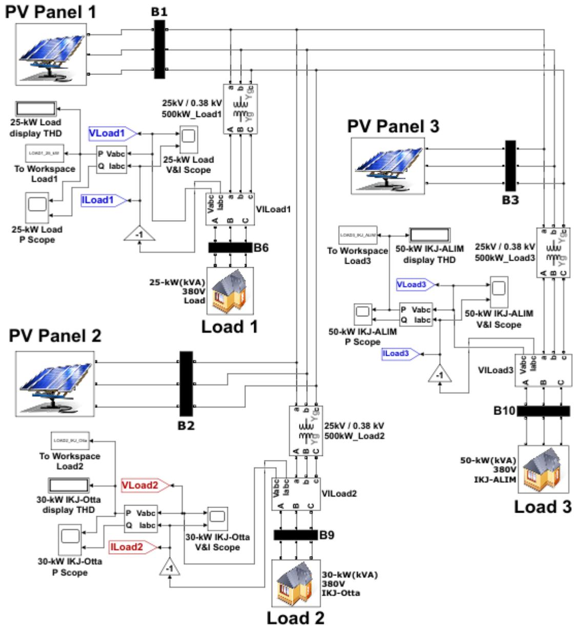
Figure 3.11: Schematics of the three photovoltaic (PV) array systems connected in series to each load centre and connected in parallel to each other
