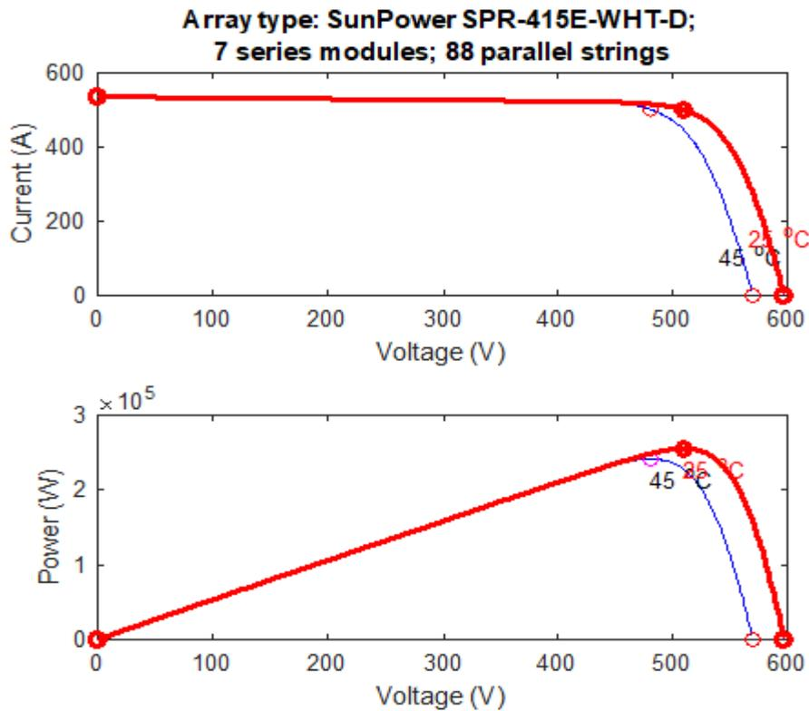
Figure 3.4: I-V and P-V graphs of the SunPower SPR-415E-WHT-D PV array
