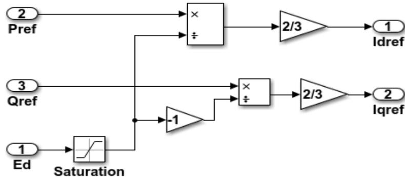
Figure 3.8: Schematics of the P-Q control subsystem
