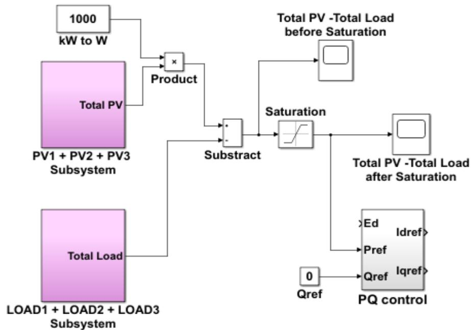
Figure 3.13: Schematics of how the logic control is integrated into the P-Q control system
