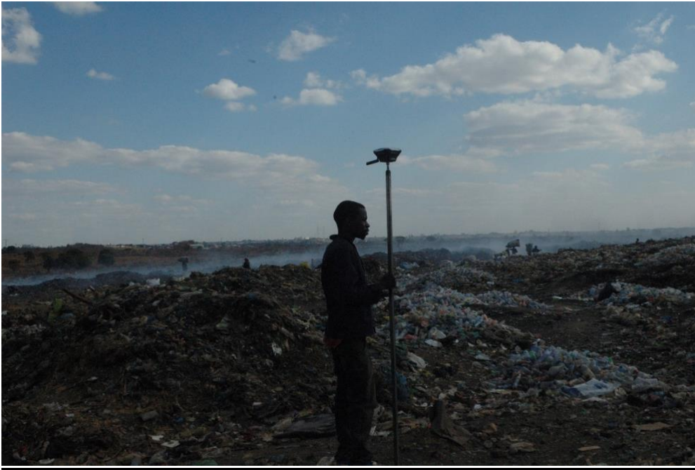
Figure 5:3: An EMLID Rover is held in place to collect GCP at Chunga Landfill.
