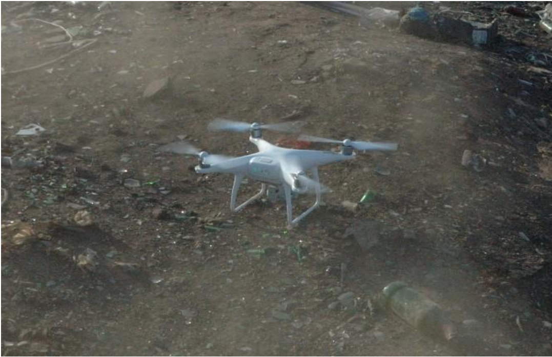
Figure 5:2: Phantom 4 (UAV) used for image acquisition at Chunga landfill.
