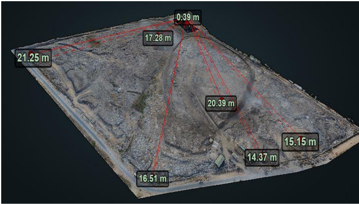
Figure 5.9: Terrain elevation at Chunga landfill based on the lowest point at the landfill (Zone F) and NOT measured in relation to sea level.
