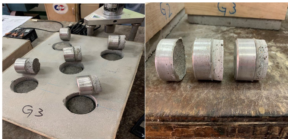
Figure 4. Pull off mortar samples after 28 days of age (Mix 7).
