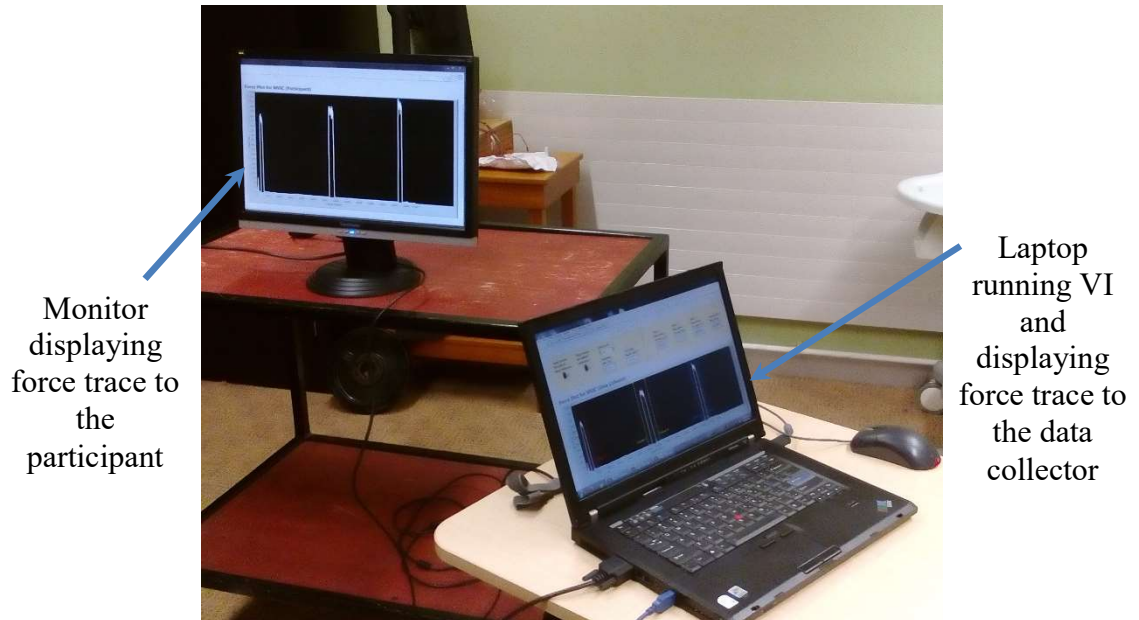
Figure 4.5 Laptop and extended monitor displaying generated force trace to both the data collector and participant.
