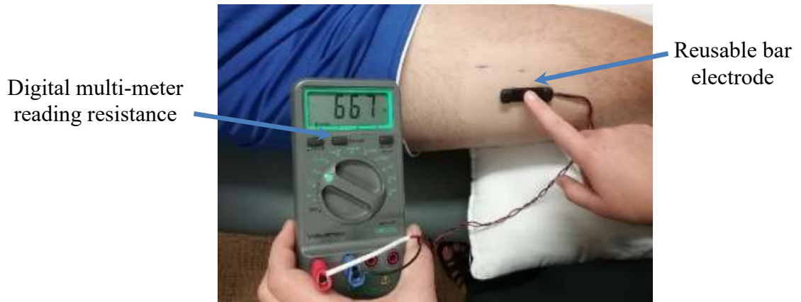
Figure 4.8 Measuring the skin resistance using a multi-meter.
