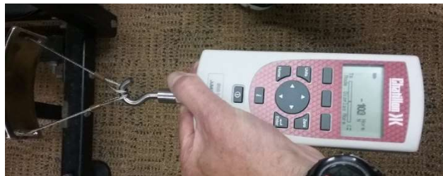
Figure E.2 Force of 100 N applied to the load cell assembly using a Digital Force Gauge.
