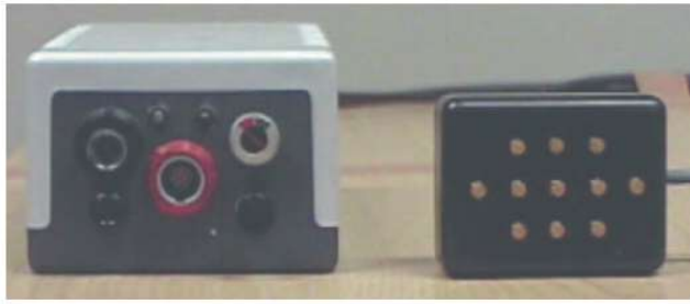
Figure 6.1 Three-channel Laplacian electrode (right) and amplifier/power supplier (left) used in pilot study [37, 38].
