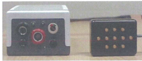
Fig. 2. Three-channel Laplacian electrode (right) and amplifier (left) used for data collection of sEMG signals from the vastus medialis muscle of the quadriceps.
