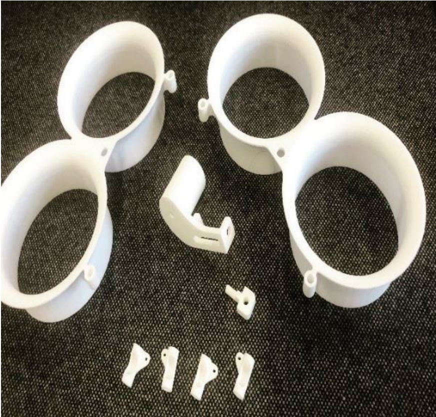
Figure 2: (Cleveland, 2022) SLS 3-D printed componentry [photograph]
