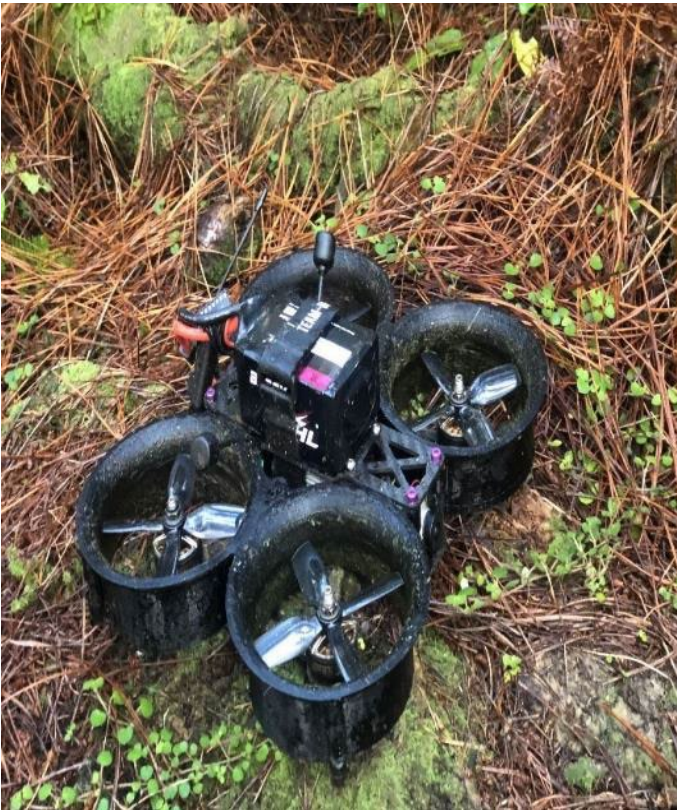
Figure 3: (Cleveland, 2022) TPU 3-D printed componentry fitted on the drone with cut down propellers [photograph]
