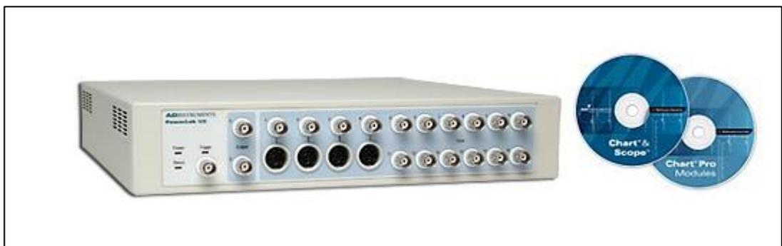
*Figure 4.9. ADInstruments PowerLab 16/30. Input from signal conditioners and transducers is possible with 16 available channels to select. Coaxial cable and pod ports are provided for connectors. The DLP 2.5 (tracheal pressure data source) and Honeywell transducer (oesophageal pressure data source) are connected to ports 1 and 7 of the PowerLab system board. Output of signals is sent to LabChart software for further processing.*
