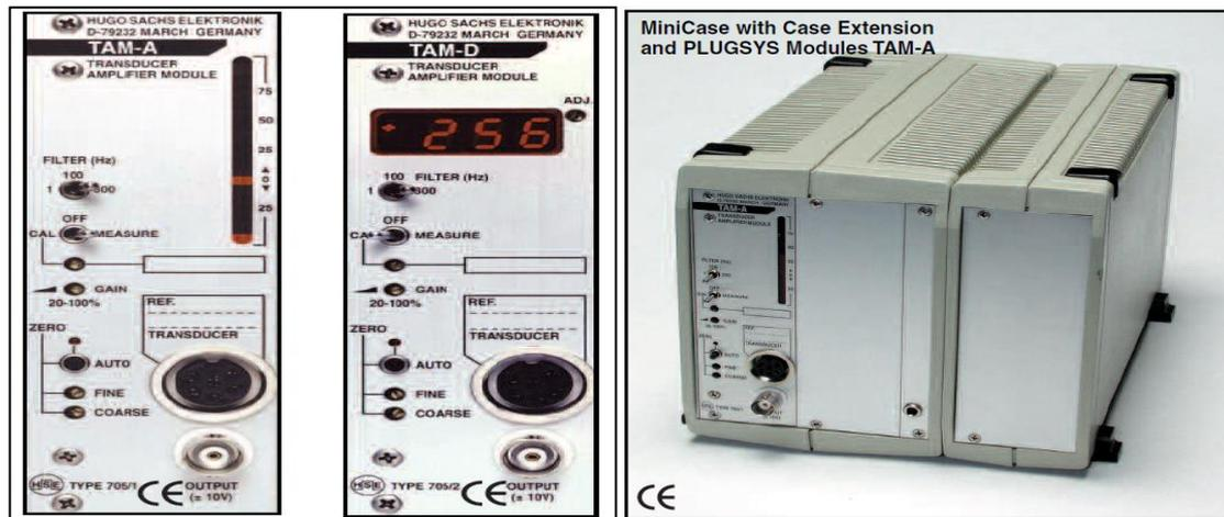
Figure 4.6. TAM-A transducer amplifier module and its PLUGSYS Minicase. The minicase contains the amplifier module, the power supply for the amplifier, and has a second slot available for installation of an additional transducer amplifier module. The connection cable from the DLP 2.5 (shown in Fig. 4.5(d)) locks into the 6-pin socket of the TAM-A module.
