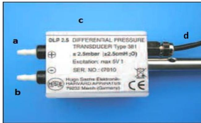
Figure 4.5. Differential Low-Pressure Transducer DLP 2.5. The key functional areas of the component are listed as follows: a) Inlet for oral-level pressure signal, b) Inlet for atmospheric pressure signal, c) Body of the differential pressure transducer, d) Connection cable from DLP to signal amplifier. Dedicated tubes from the pneumotachometer's outlets (Figure 4.3, b and c) are connected to DLP inlets a and b respectively, allowing for measurement of low pressure signals during protocols.
