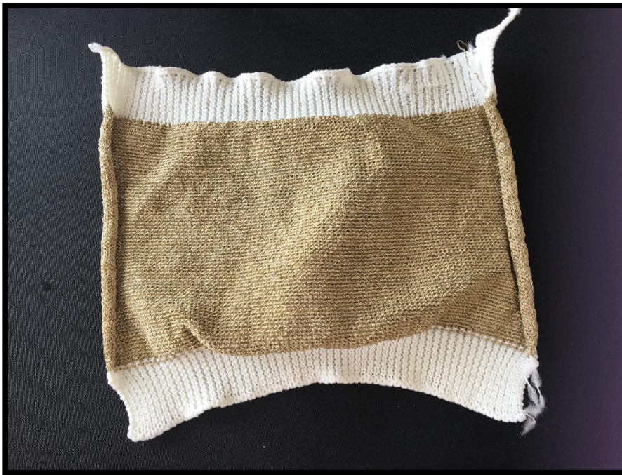
Figure 38: Stainless steel sample curling edges
