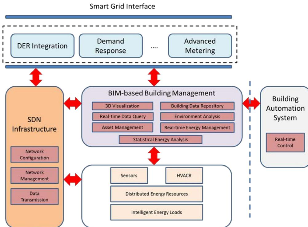
**Figure 4.13. Smart-Grid-Ready Building with BIM and SDN**
