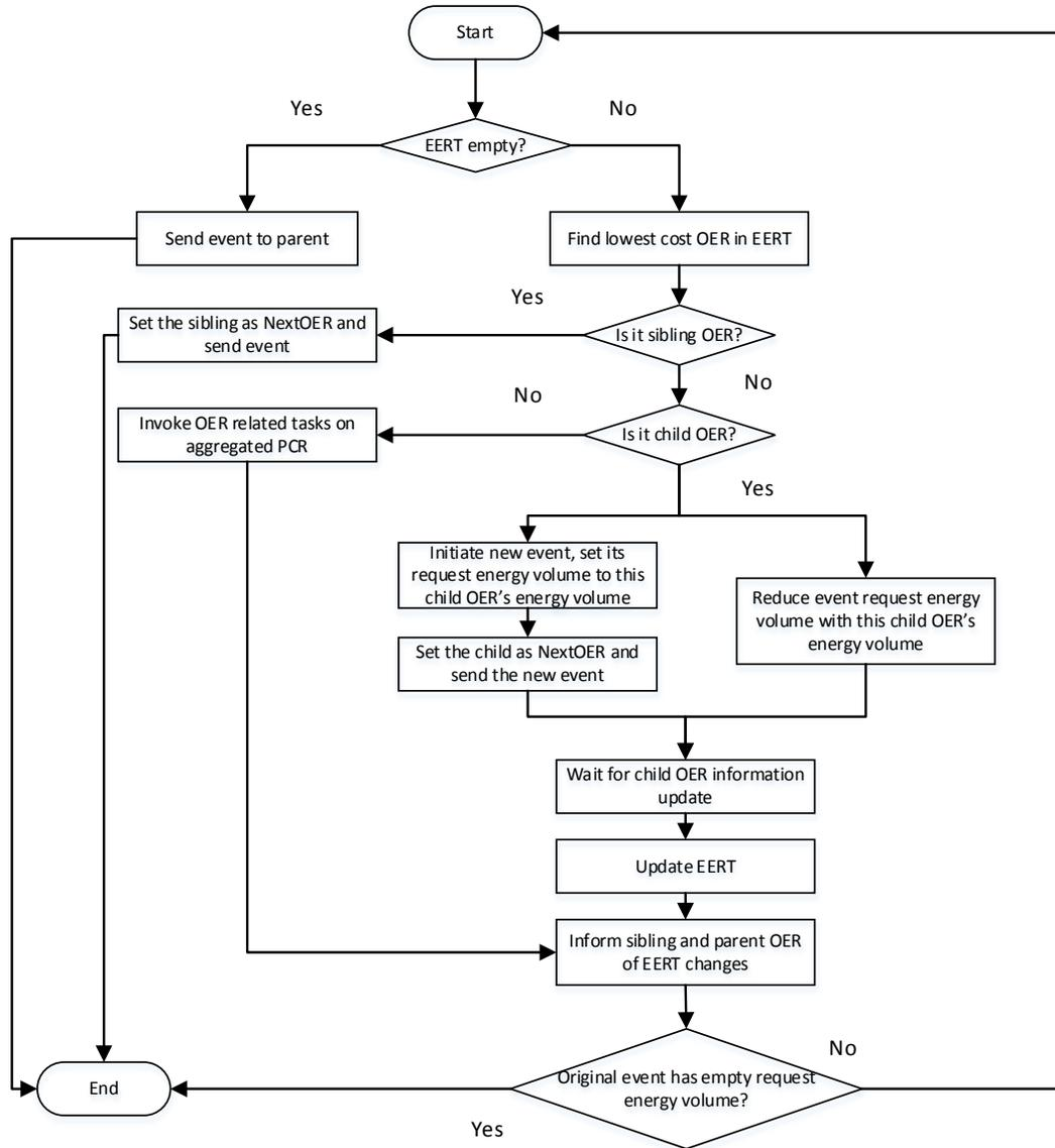
Figure 5.7 Energy Event Routing (Algorithm 2)
