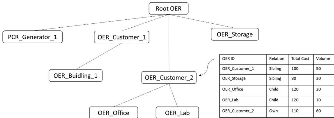
**Figure 5.5 Example of VPP Tree structure and Energy Event Routing Table**
