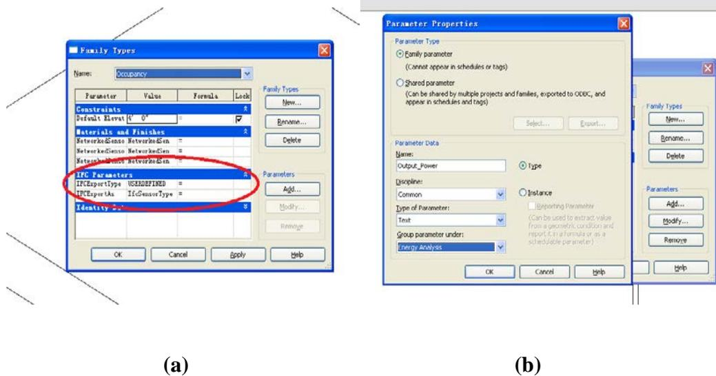
**Figure 4.2 (a) Extending BIM design using “IFC shared parameter”. (b) Adding new parameter properties in Revit**
