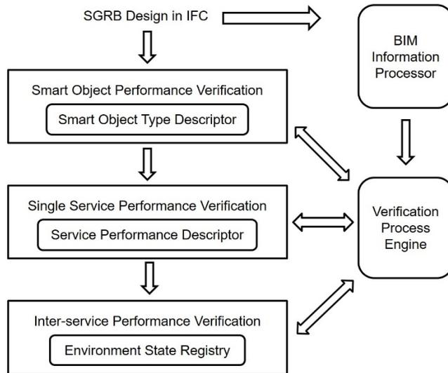
**Figure 4.5 Design Verification Framework for Smart-Grid-Ready Buildings with BIM**
