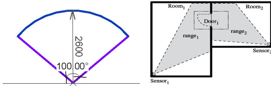
**Figure 4.3 (a) Example of range space of a sensor with range radius of 2.6m and range angle of 100 degrees. (b) The door's operational space should be within the range space of the two monitoring sensors.**
