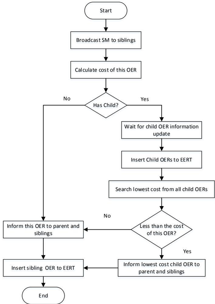
**Figure 5.6 Energy Event Routing Table Initialization (Algorithm 1)**
