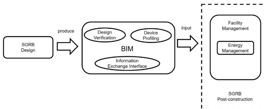
**Figure 4.1 Role of BIM in Smart-Grid-Ready Buildings**
