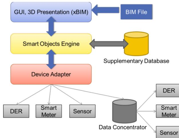
**Figure 4.9 BIM-based Energy Management Platform Software Architecture**
