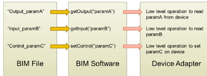
**Figure 4.8 Mapping from BIM file to Software Information Interface Programming**
