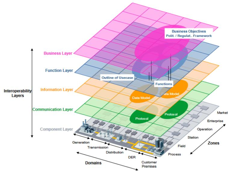
**Figure 3.3 Smart Grid Architecture Model**
