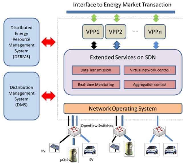
**Figure 4.12 DER Aggregation with SDN**
