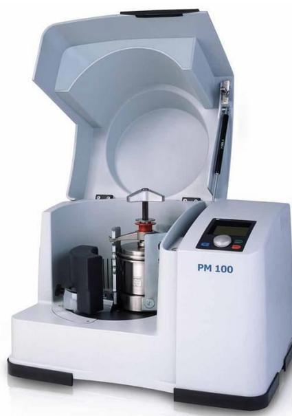
*Figure 24 – Retsch PM-100 Planetary Ball Mill (Retsch GmbH, 2016)*
