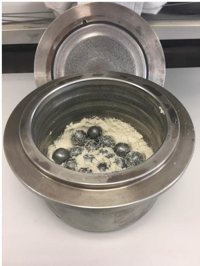
*Figure 25 – 20 Steel balls 20 mm in diameter in the milling jar with quartz.*
