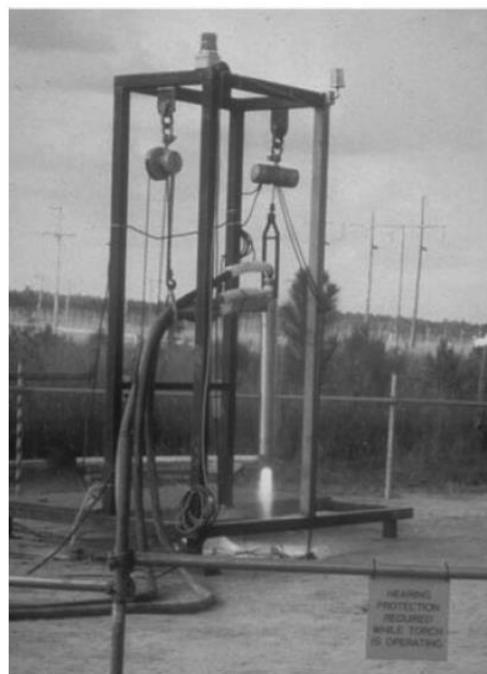
Figure 8 - One-Megawatt Plasma Torch Prior to Insertion into Borehole in the Test at the Savannah River Site (Fox, Circeo, & Martin, 2001)
