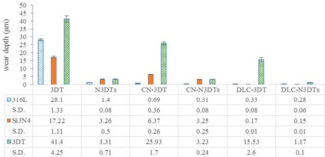
Fig. 2.34 Wear depths of all specimens when sliding against 316L, Si<sub>3</sub>N<sub>4</sub> and 3DT balls. (S.D. denotes standard deviation) [74].
