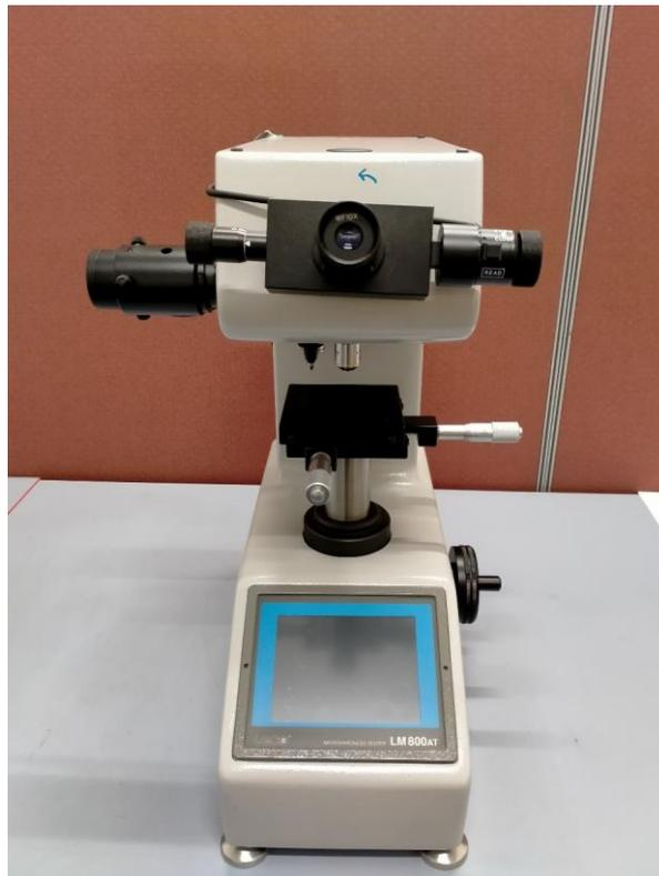
Fig. 3.1 Micro-hardness tester.
