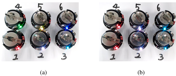
Fig. 16. Kilobots demo illustration: (a) Channel allocation complete; (b) Rendezvous complete.
