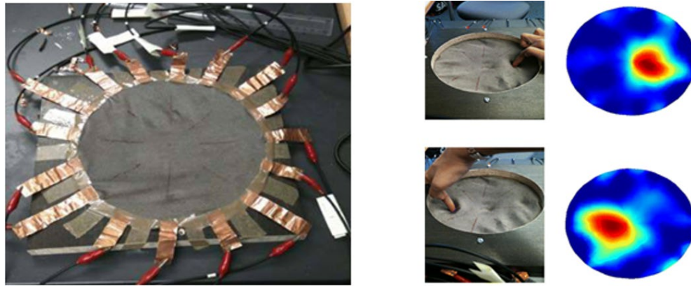
Figure 2-25 EIT is applied to a piece of conductive fabrics to enable pressure detection[209]. (Copyright 2012 Emerald Publishing Limited. Reused with permission).
