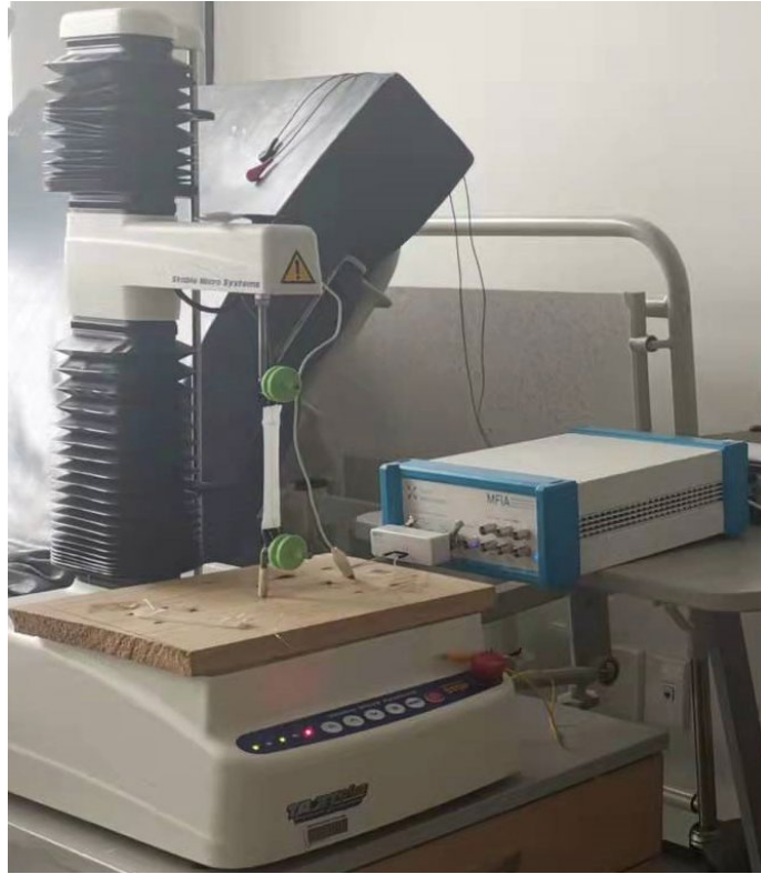
Figure 5-2 Experiment setup: a sensor was mounted to TA.XT-plus for receiving strain and was characterized by MFLA for its electrical response.
