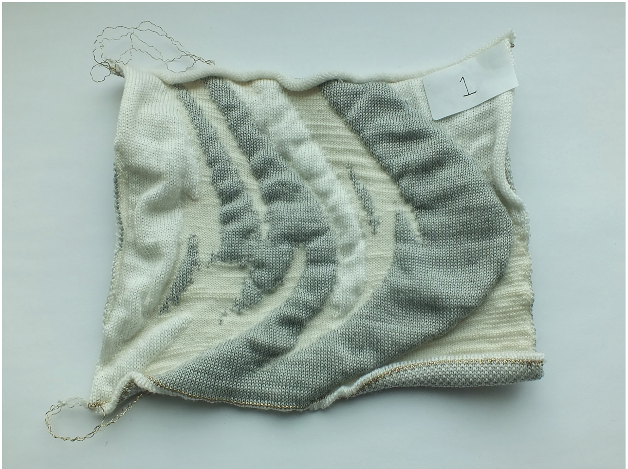
Sample One: Stainless steel / polyester yarn and merino tested for electrical response when 10 kg of force was applied.
