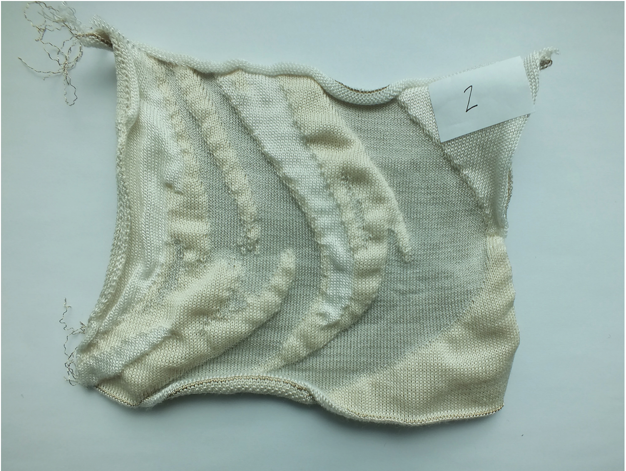
Sample Two: Silk / Steel and Seacell yarn tested for electrical response when 10 kg of force was applied.
