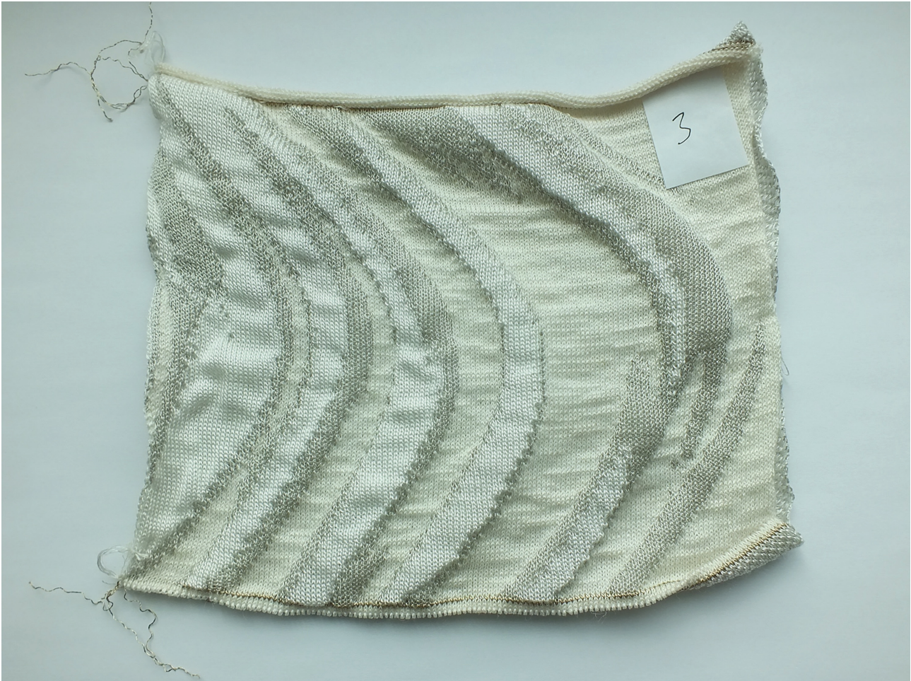
Sample Three: Silk / Steel and Bamboo yarn, tested for electrical response when 10 kg of force was applied.
