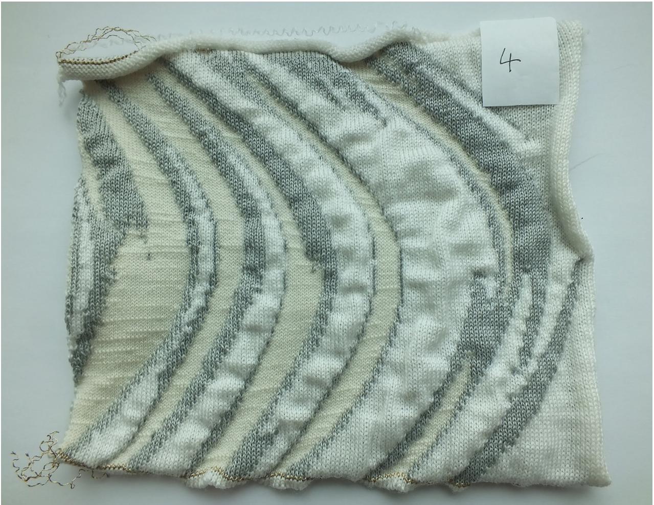
Sample Four: Stainless steel / polyester yarn and merino tested for electrical response when 10 kg of force was applied.
