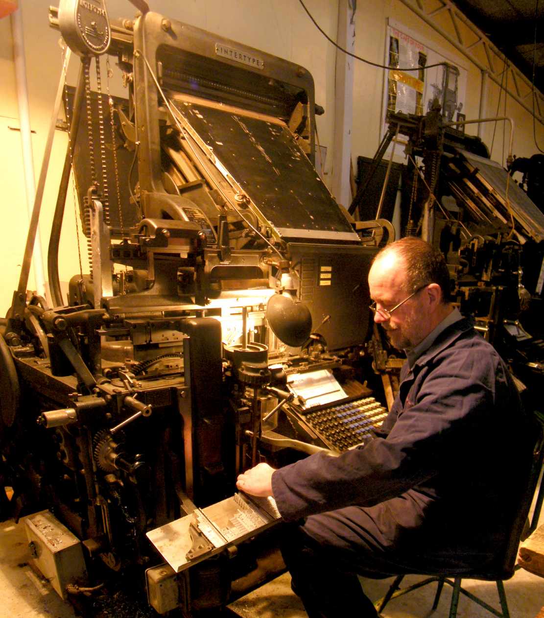
Figure 70: Terry Foster setting lead type using Intertype type casting machine for the Requiem piece.
