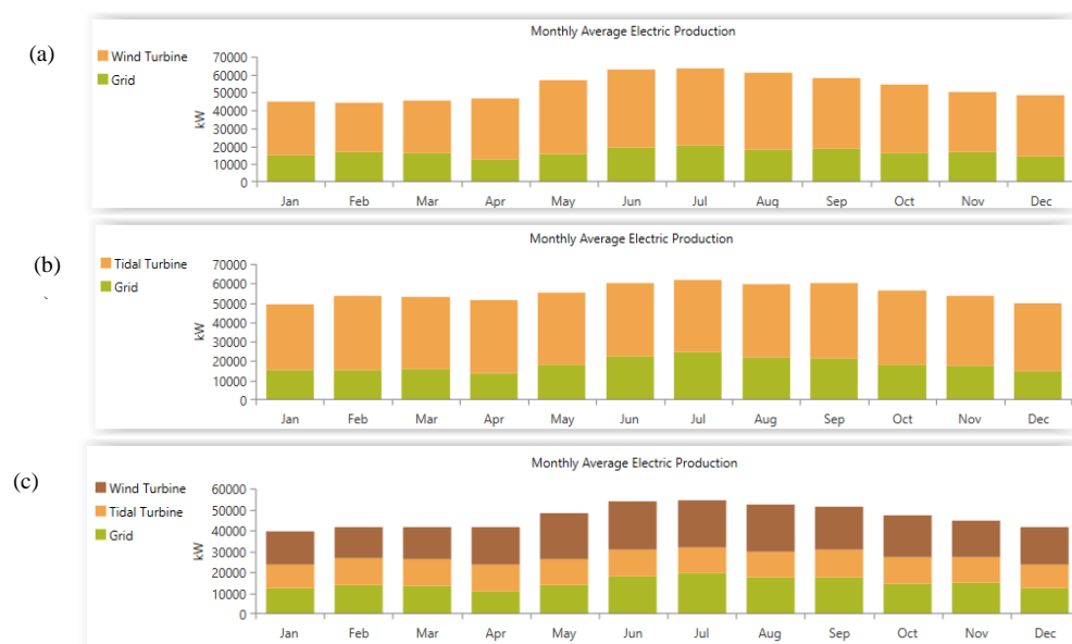
Figure 5-40: Monthly average output power for (a) 36W, (b) 113T, (c) 19W+38T.
