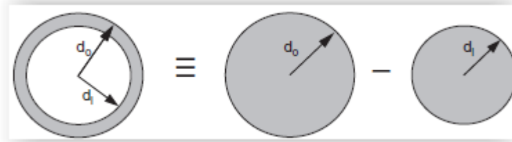
Figure D-37: Plastic moment of a hollow section estimation [160].
