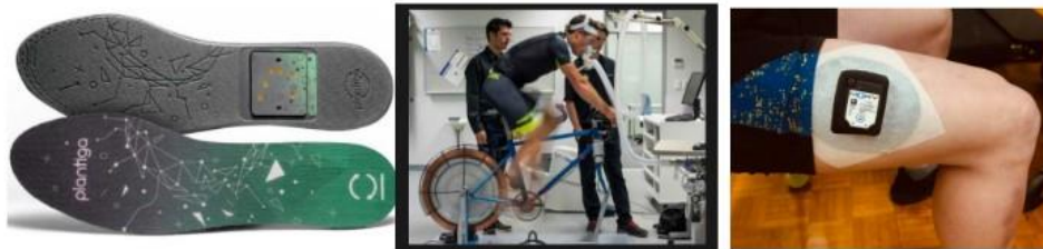
Figure 1 (from left to right): Plantiga shoe inserts, Parvo TrueOne metabolic cart, and Moxy Monitor.
