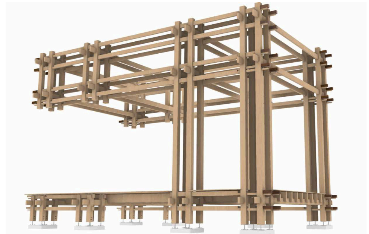
Figure 88. Final Torii Pathway structure developed with the adjustable Nuki joint system.
