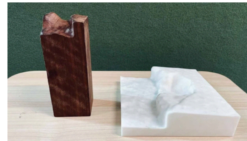
Figure 70. Tectonic model demonstrating the relationship between a CNC-milled Ishibadate-inspired timber connection and a 3D-printed façade model.
