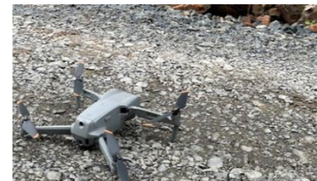
Figure 76. DJI Mavic Air 2 drone used to capture aerial photographs for photogrammetric modelling.
