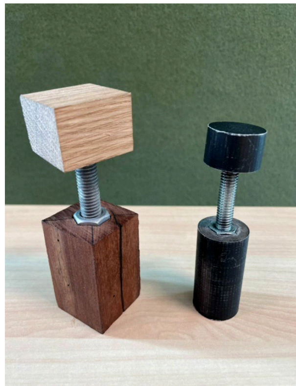
Figure 87. Prototype of adjustable extension component of the Nuki joint system.
