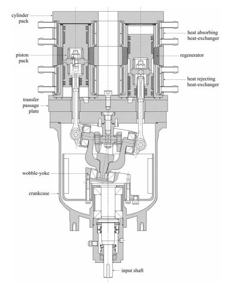
Figure 5. Cross-sectional general assembly drawing of DH1 heat-pump/refrigerator experimental rig in a  $4-\alpha$  double-acting configuration (some components removed for clarity).
