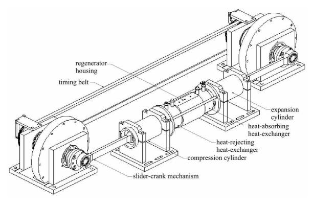
Figure 6. General assembly drawing of MAG1 regenerator test rig.
