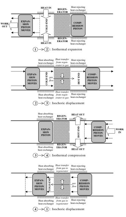
Figure 3. Thermodynamic processes in the ideal Stirling-cycle refrigerator or heat-pump as shown on a simplified  $\alpha$ -configuration machine.
