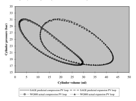
Figure 4. Actual and SAGE predicted WG800 cylinder pressure with variation in volume.
