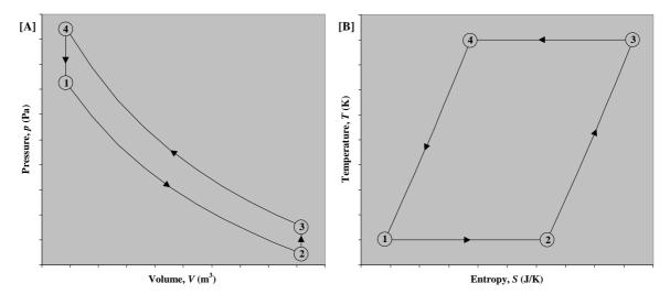
Figure 2. Thermodynamic processes in the ideal Stirling-cycle refrigerator or heat-pump. (A) Pressurevolume diagram. (B) Temperature-entropy diagram.
