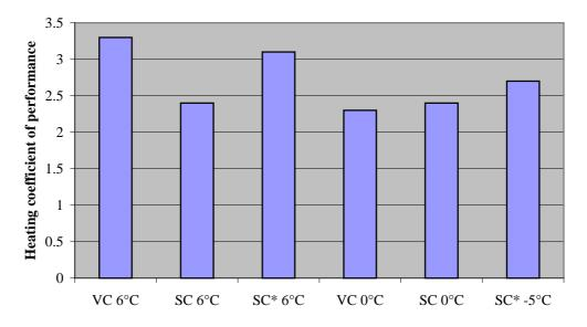
Figure 7. Some results from the Stirling-cycle heat-pump development programme.
