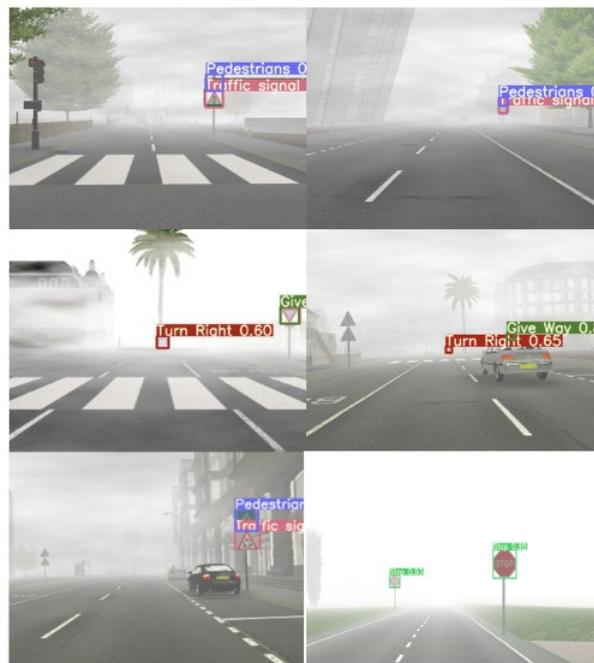
Figure 4.7: TSR results regarding the improved Faster R-CNN model in foggy scenes
