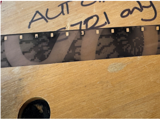
Figure 10. 16mm film shows the imprint of scissors left in the exposure area.
