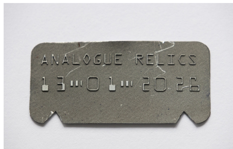
Figure 24. Aluminium plate embossing created by removal of metal from around the characters.
