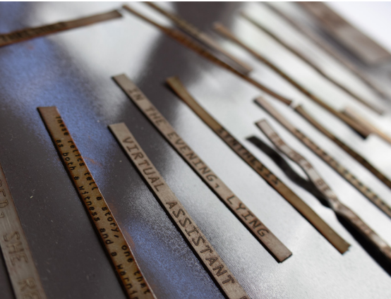
Figure 30. Shows various grades and thicknesses of steel tested with the fibre laser.
