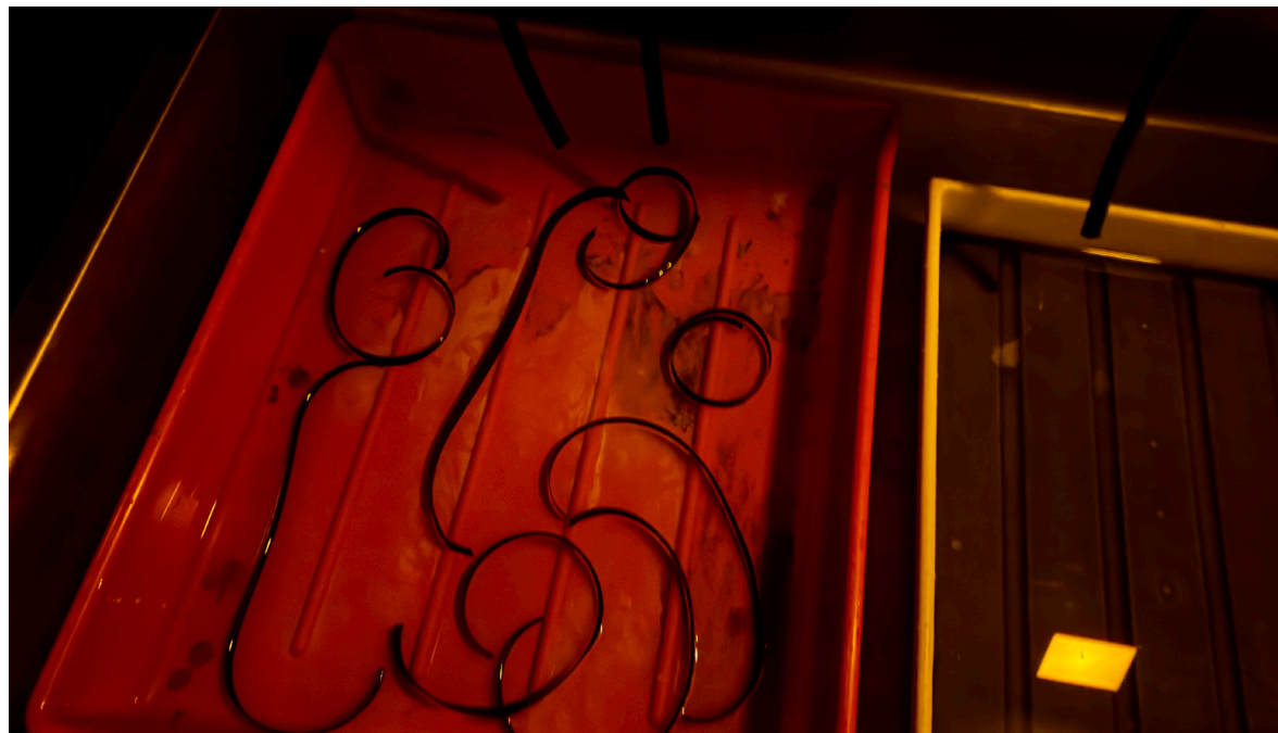
Figure 11. Darkroom developing process. Strips of 16mm film sit in a water bath, for post-fix rinse. The image is now stable so it can be exposed to light. This is the last step before applying wetting agent.
