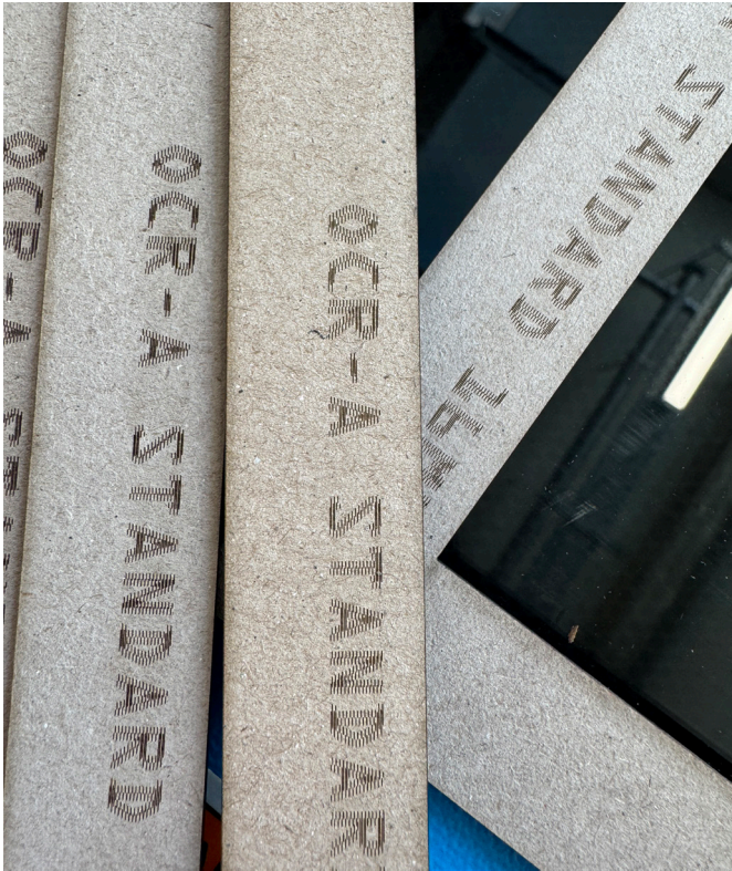
Miscalibration on etched text from laser cutting process
