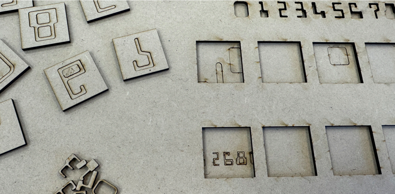
Early experiments involved laser cutting MICR Glyphs from wood.
