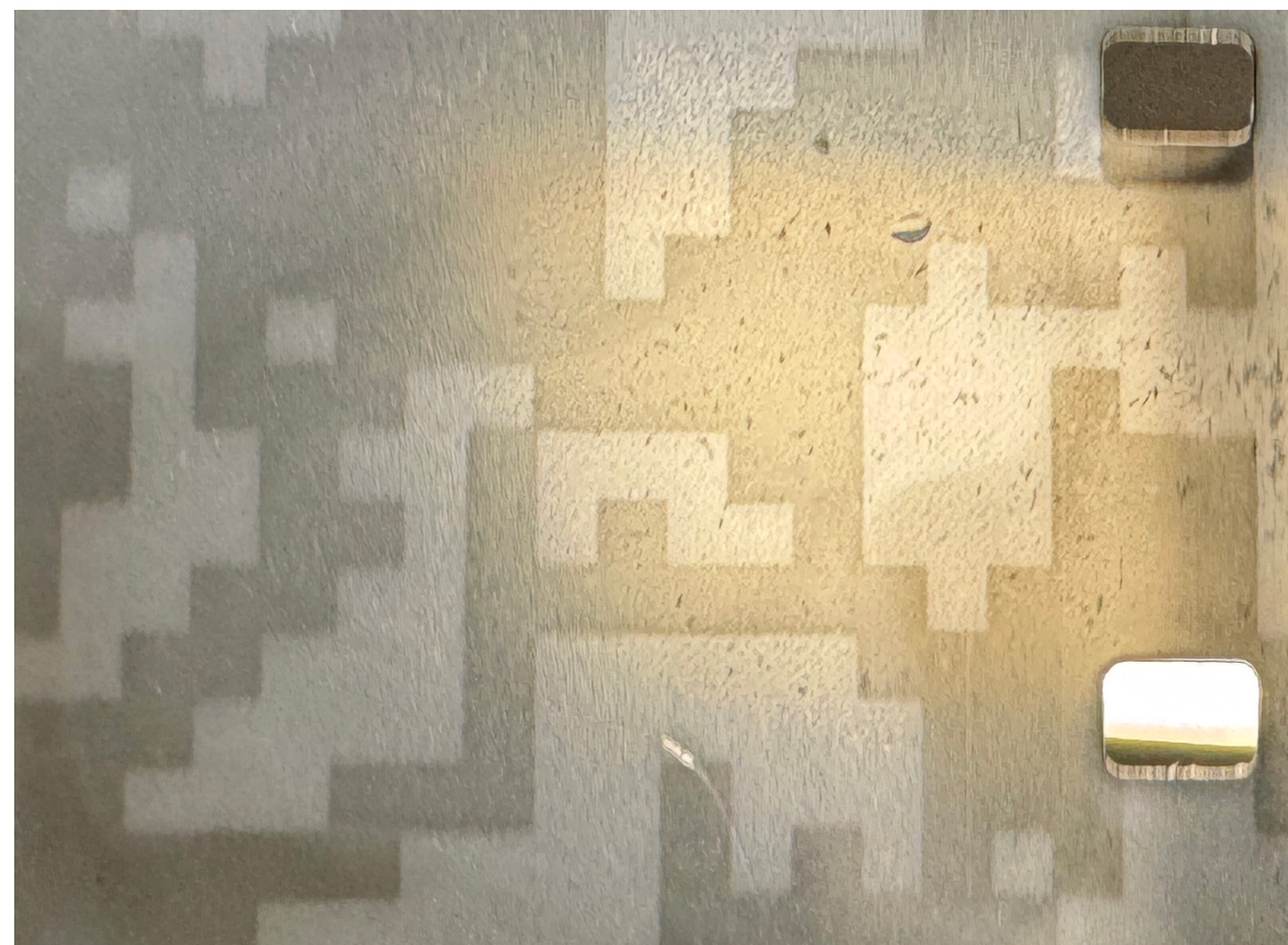
Figure 12. Post processing. The film shows traces of detritus left from the development process.
