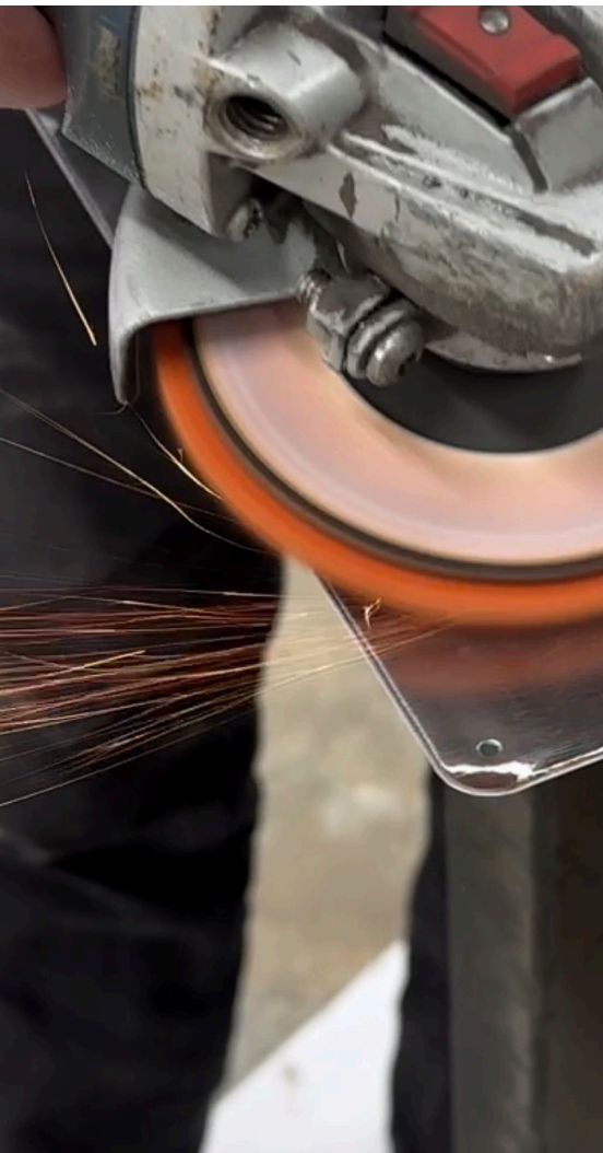
Figure 32. The bright orange sparks from the grinder test suggest that this was a form of steel.
