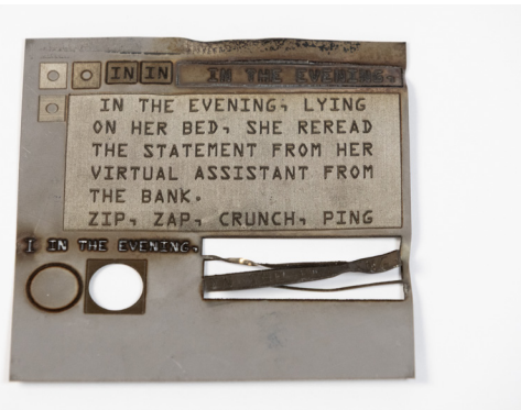
Figure 29. Steel testing plate, for laser fibre laser settings
