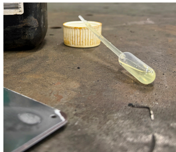
Figure 33. Acid test produced a cloudy result that cleaned the surface of the metal suggesting that it was a form of steel.
