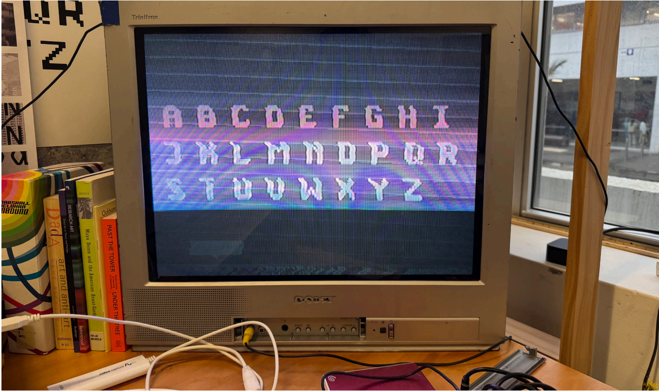
Using a CRT distorter to disrupt a typeface. The distorter is an analogue device that sits between the source signal and the CRT and allows for manipulation of the signal
