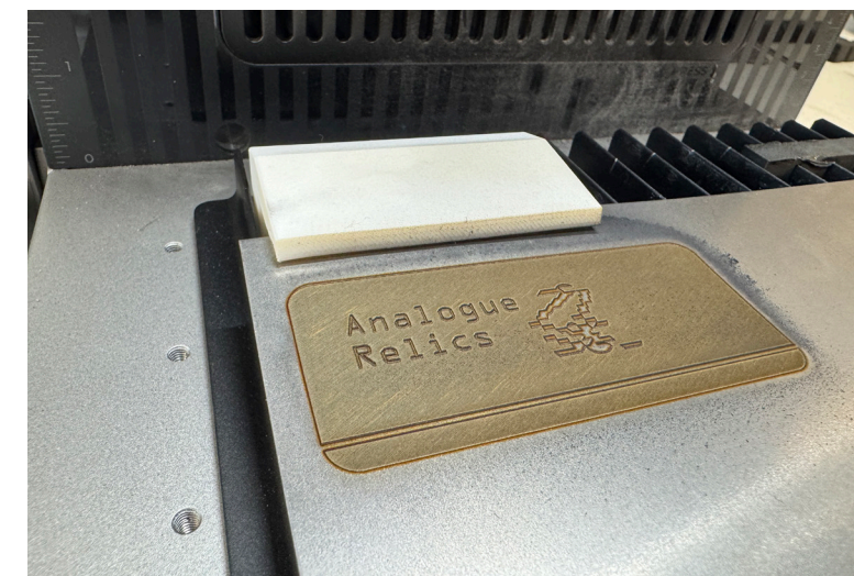
Figure 34. Jig setup to help mitigate warping and flexing of the material.
