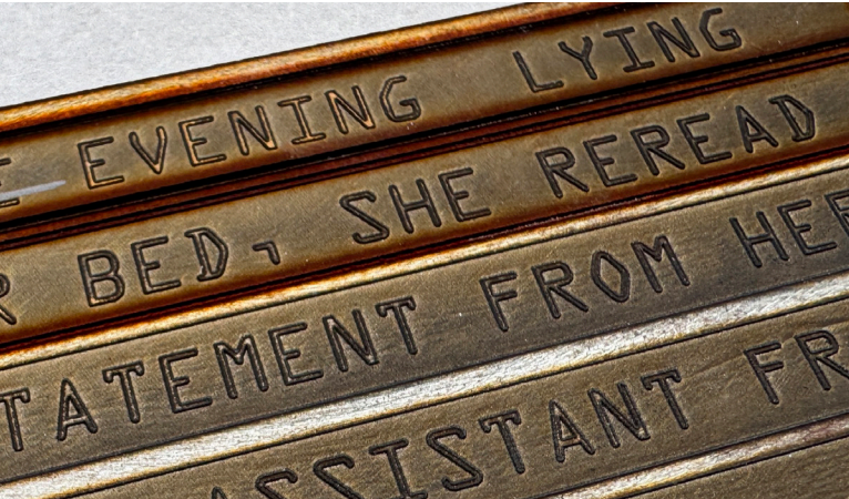
Figure 31. Shows heavy oxidation on the top two lines.
