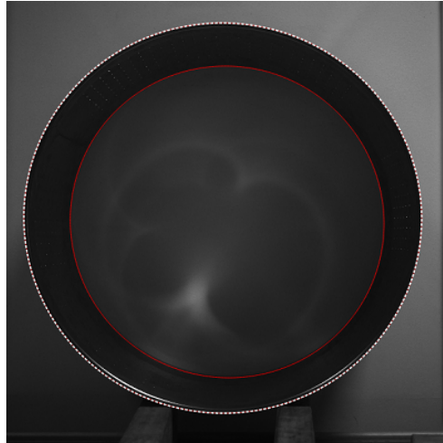
Figure 7.3: An image of the cylinder from the top with extracted edges [190].
