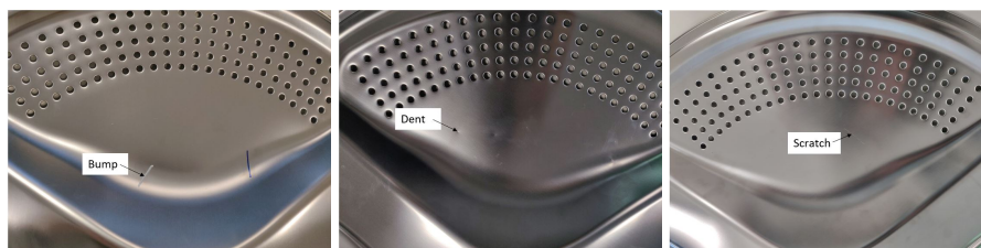
(a) An object with bumps as a defect. (b) An object with dents as a defect. (c) An object with scratches as a defect.
