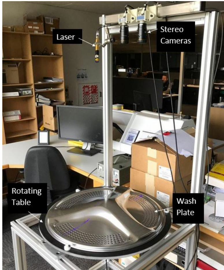
Figure 4.4: Setup of the stereo-laser system.
