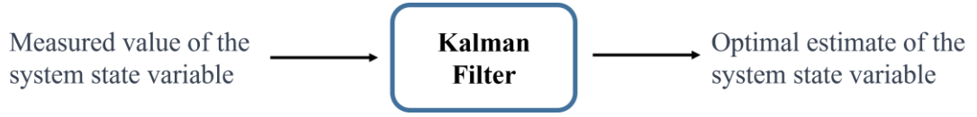
Figure 3.15: The working principle of the Kalman filter
