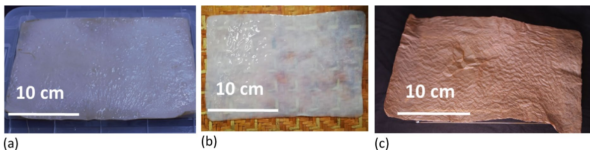
Fig. 2. BC samples: (a) washed sample (S6), (b) sample being dried in a bamboo mat (S2) and (c) dried sample (S5) ready for investigation.
