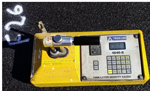
Figure 1. An NDG placed on the surface of the asphalt pavement.
