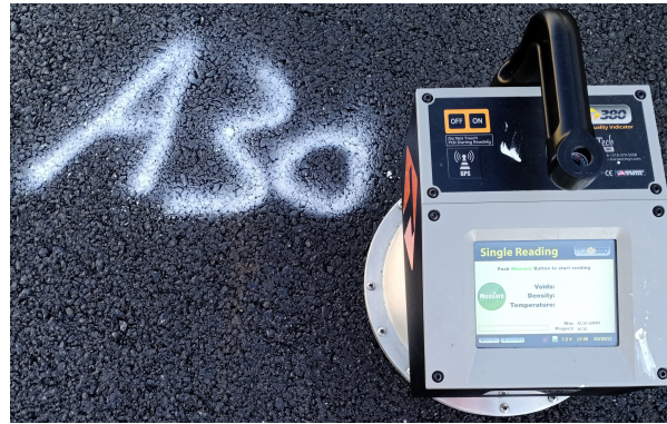
Figure 2. An EDG placed on the surface of the asphalt pavement.
