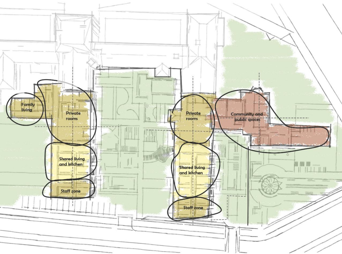
Figure 57 Zoning Option 3 - Placing private rooms directly next to public spaces violates the 'Spatial Sequencing' principle, lacking the necessary acoustic and psychological buffers for residents. Created by Author.
