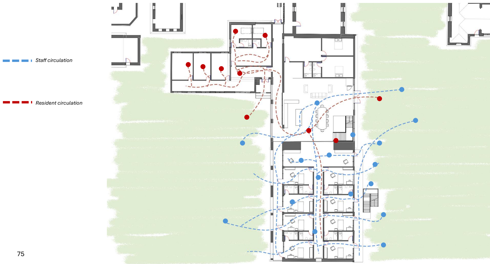
Figure 60. Circulation plan showing separated movement paths for staff and residents. Created by Author.
