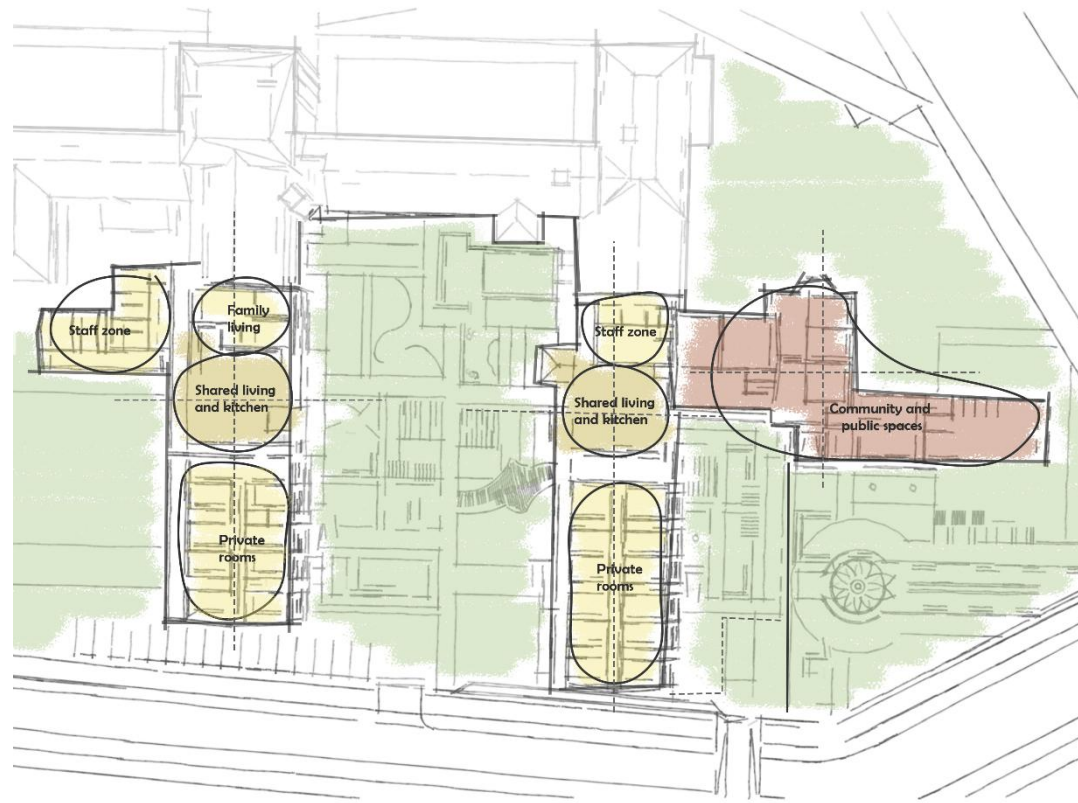
Figure 58 Zoning Option 4 - This option successfully establishes a clear hierarchy from public to private. All bedrooms receive light and views, and circulation supports gradual autonomy, making it the most resolved scheme. Created by Author.
