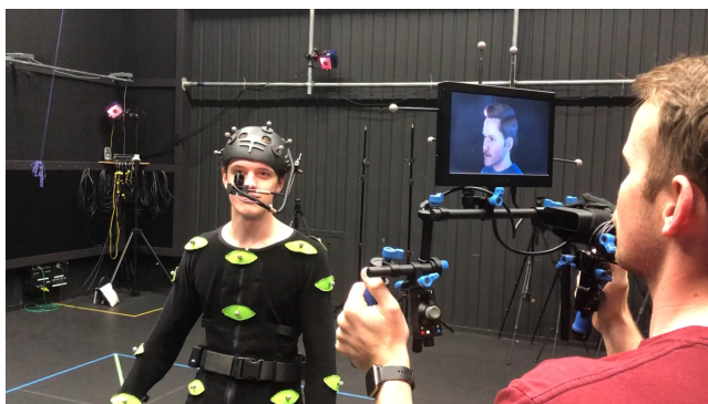
Figure 12: Live streaming body and facial motion capture data to a MetaHuman character in Unreal Engine. Live stream viewed through tracked virtual camera.
