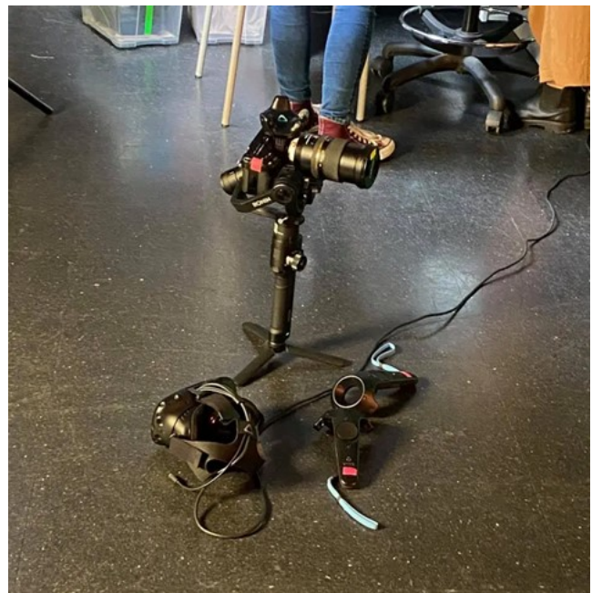
Figure 3: VIVE tracker is attached to the camera which is mounted to a gimbal. The tracker captures camera movements for live feedback.
