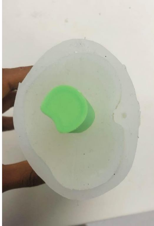
Figure 102 The assembled anatomical upper arm phantom
