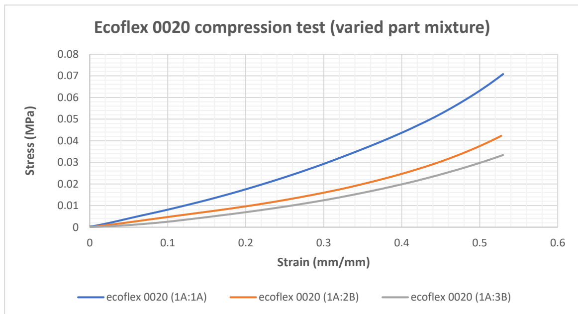
Figure 80 Stress vs Strain relationship of Ecoflex-0020 (1A:1B), Ecoflex-0020 (1A:2B), Ecoflex-0020 (1A:3B) for working strain range under compression loading
