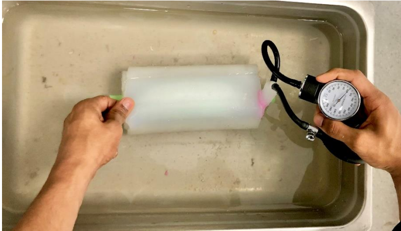
Figure 104 Brachial artery pressure test for leakages
