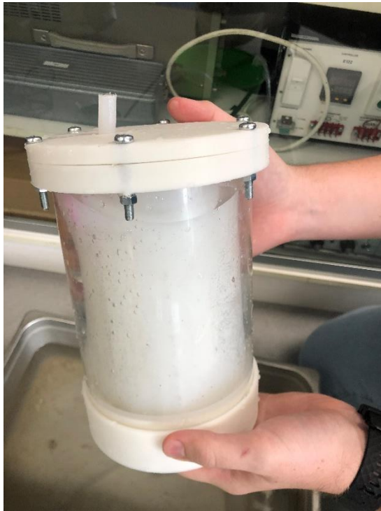
Figure 110 Test rig filled with water to emulate CP on the outer surface of the arm phantom
