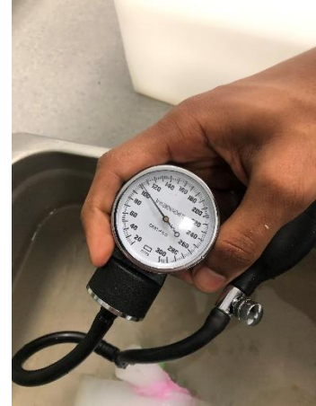
Figure 105 Stable reading on sphygmomanometer suggesting pressure loss.
