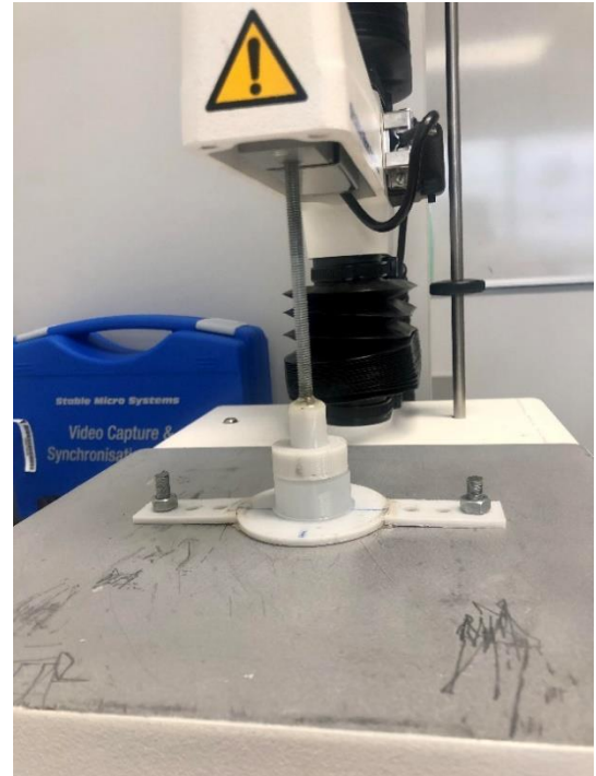
Figure 78 Compression test set up on Texture Analyser
