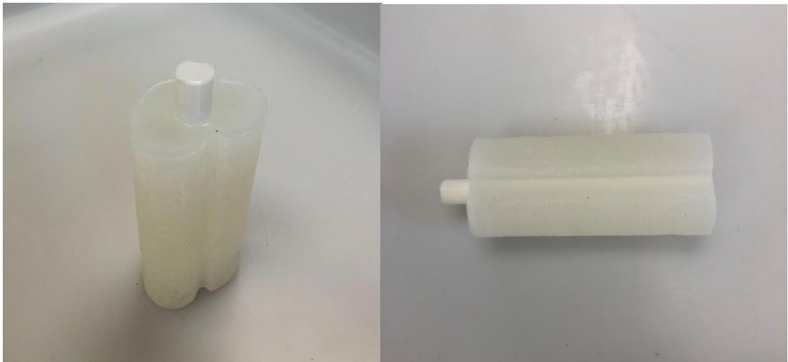
Figure 101 Isometric (left) and a lateral (right) view of the cast muscle layer
