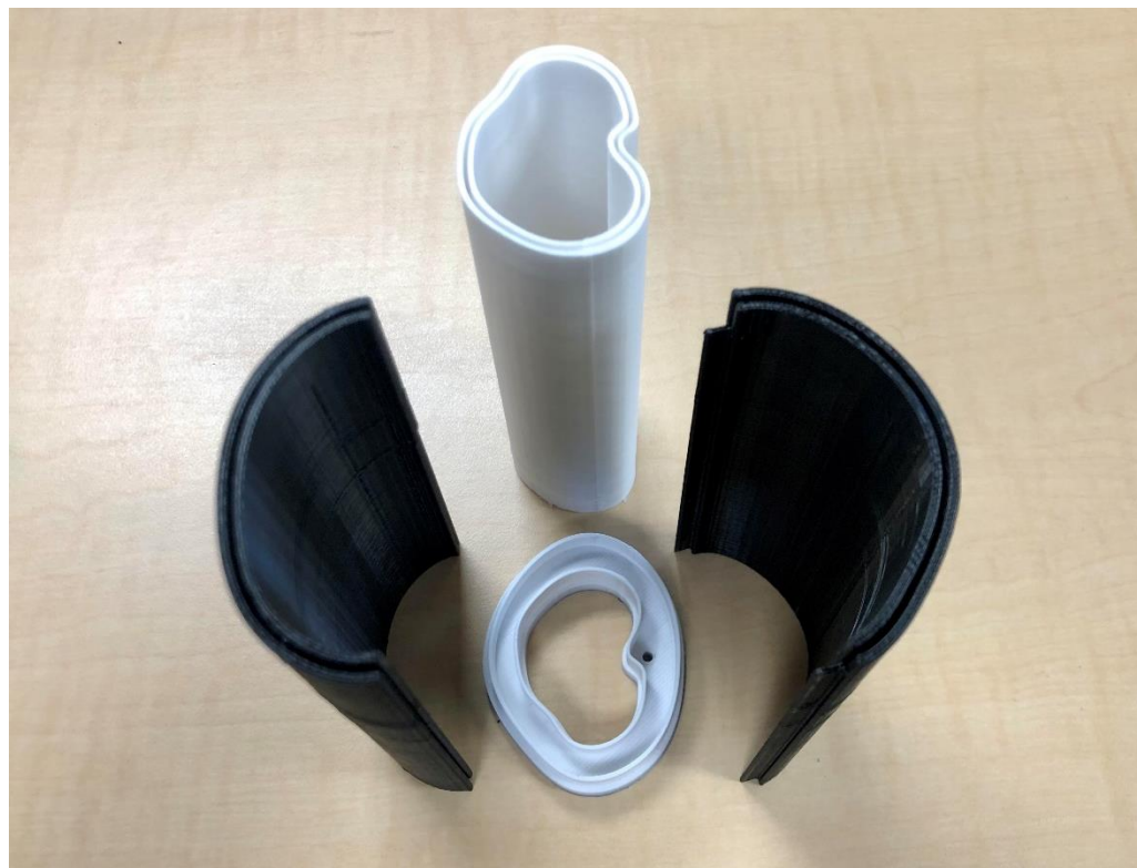
Figure 94 1:2 3D printed mould assembly for testing.
