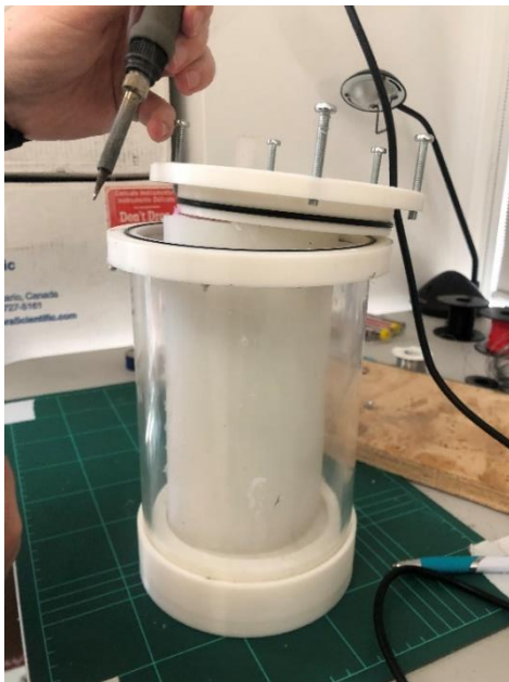
Figure 108 Openable 3D printed lid on the test rig
