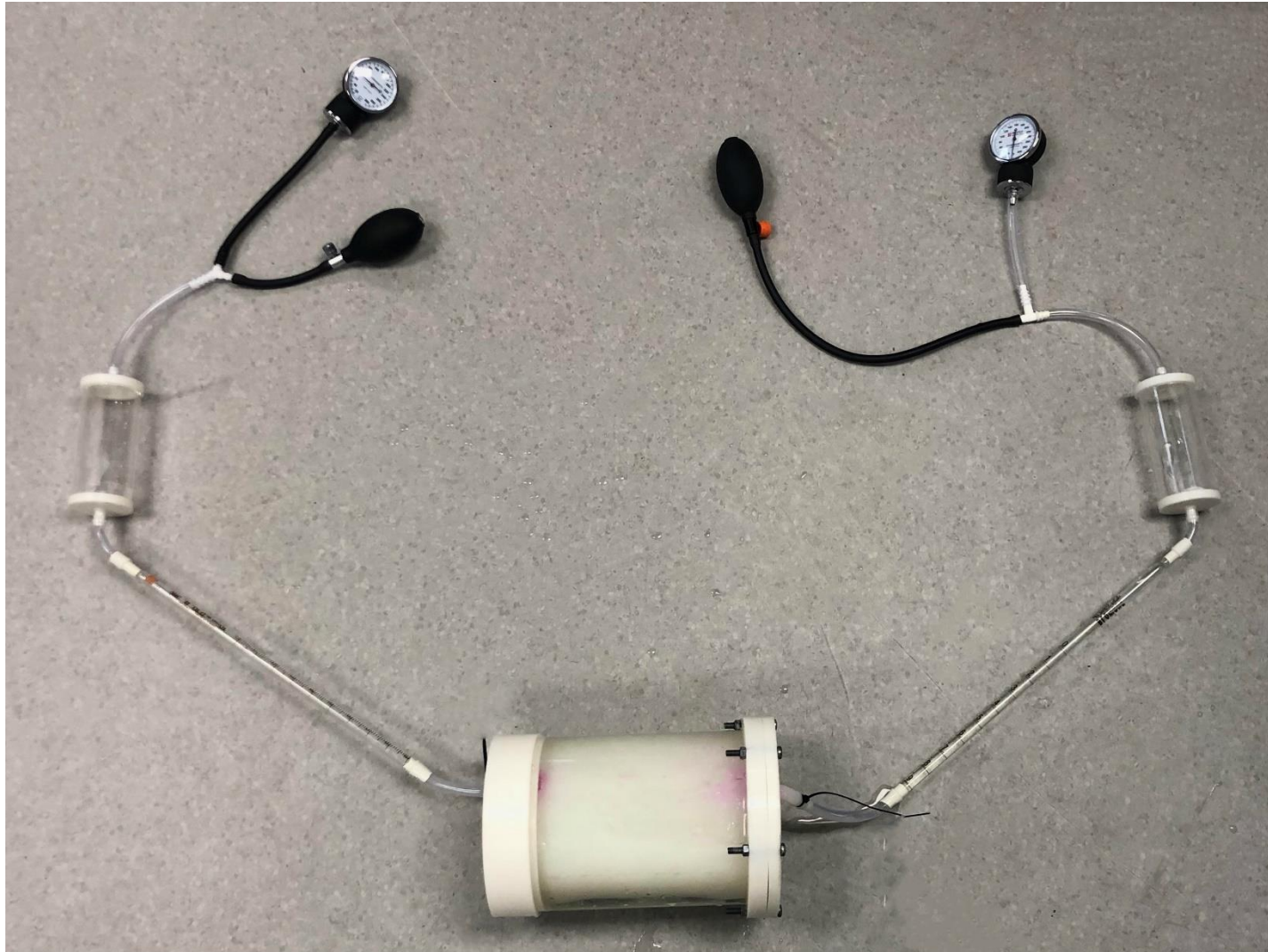
Figure 113 Test rig setup to obtain the pressure-volume change relationship in the upper arm phantom during NIBP measurement.
