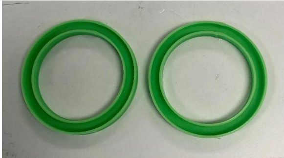
Figure 69 3D printed Moulds for ring specimens
