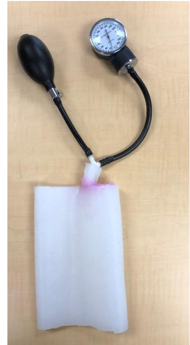
Figure 103 Attachment of sphygmomanometer and a hand pump with the brachial artery
