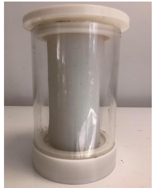
Figure 109 The upper arm phantom enclosed inside the test rig
