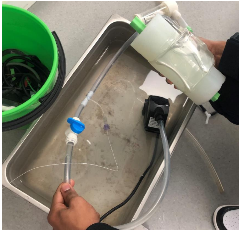
Figure 106 Preliminary test rig setup check using a clear cuff and a catheter
