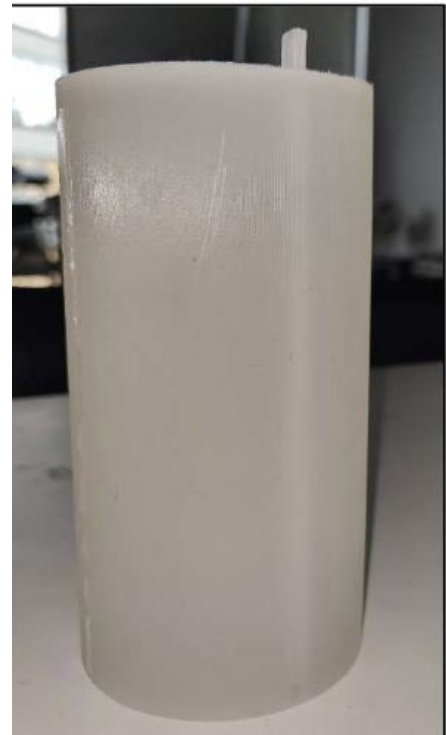
Figure 21 Cylindrical arm phantom with a separate arterial wall developed using Platsil-00 (Subburaj, 2020).
