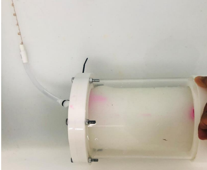
Figure 111 Pipette connected at the end of the brachial artery to measure volume change
