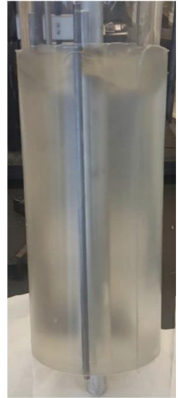
Figure 19 Simple cylindrical arm phantom fabricated using 15% SEBS gel (Anderson-Jackson, 2016)
