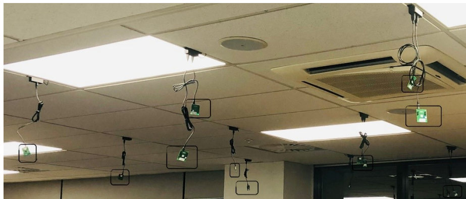
Figure 6-1 Physical network set-up in SeNSE lab (a) TI CC2538 leaf nodes.
