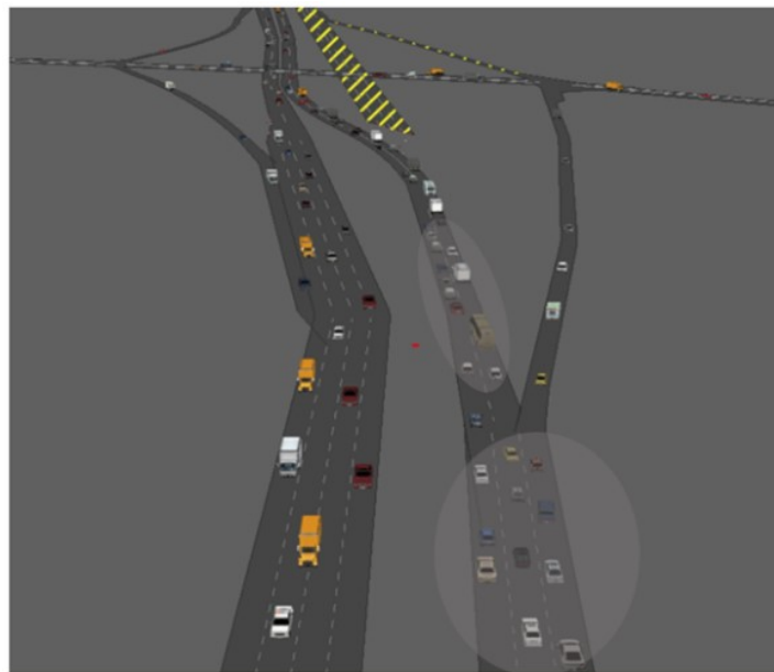
Figure 1-4 Traffic grouping scenario on a typical highway.
