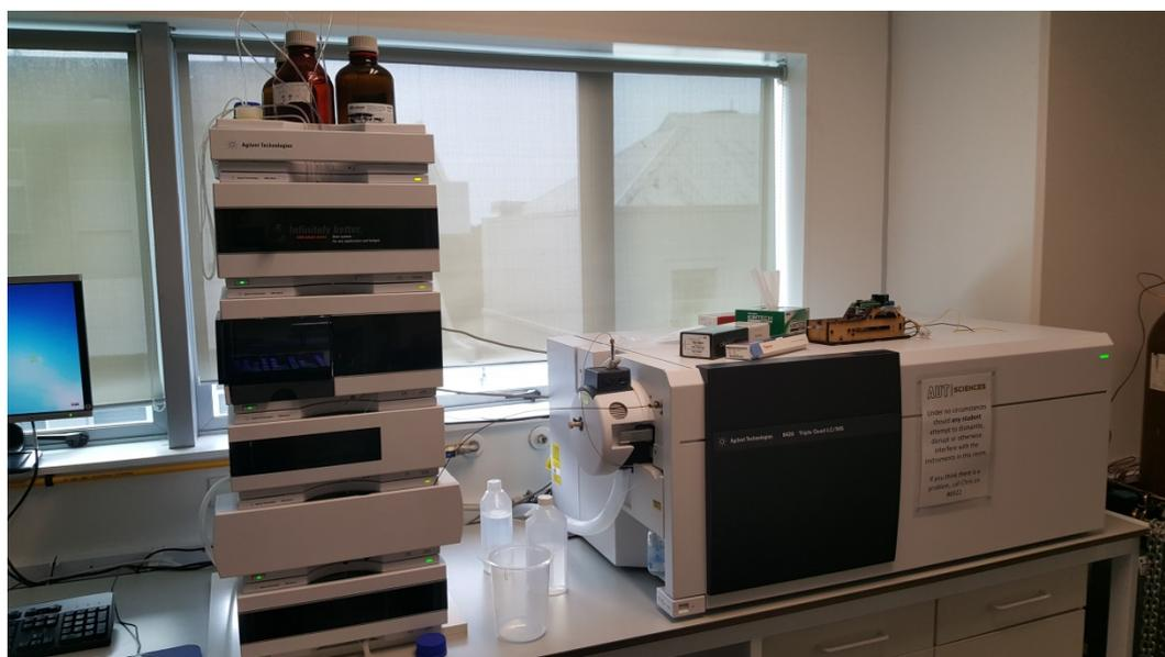
Figure 6. A photo of Agilent 6420 Triple Quad LC/MS used in this project.
