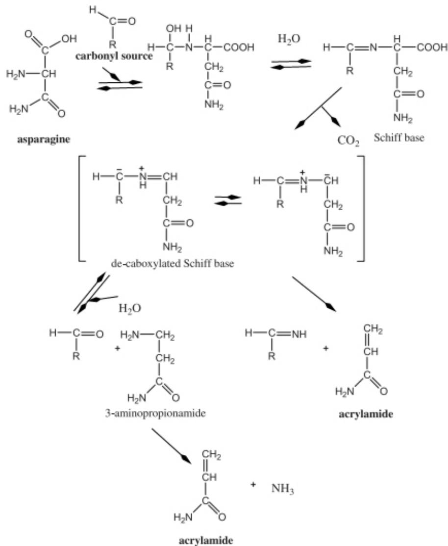
Figure 2. Schematic diagram illustrating the mechanism of acrylamide formation through Maillard reaction (Zyzak et al., 2003)
