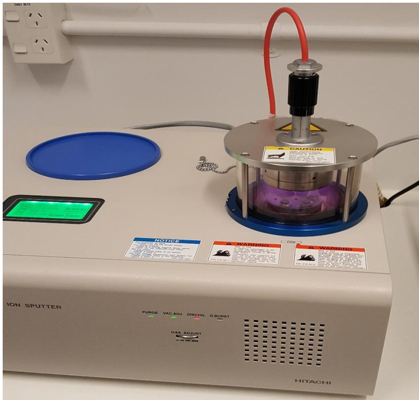
Figure 8. The ion sputter coater for SEM (Hitachi E-1045).
