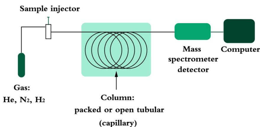
Figure 3. A schematic diagram of a typical GC-MS unit.
