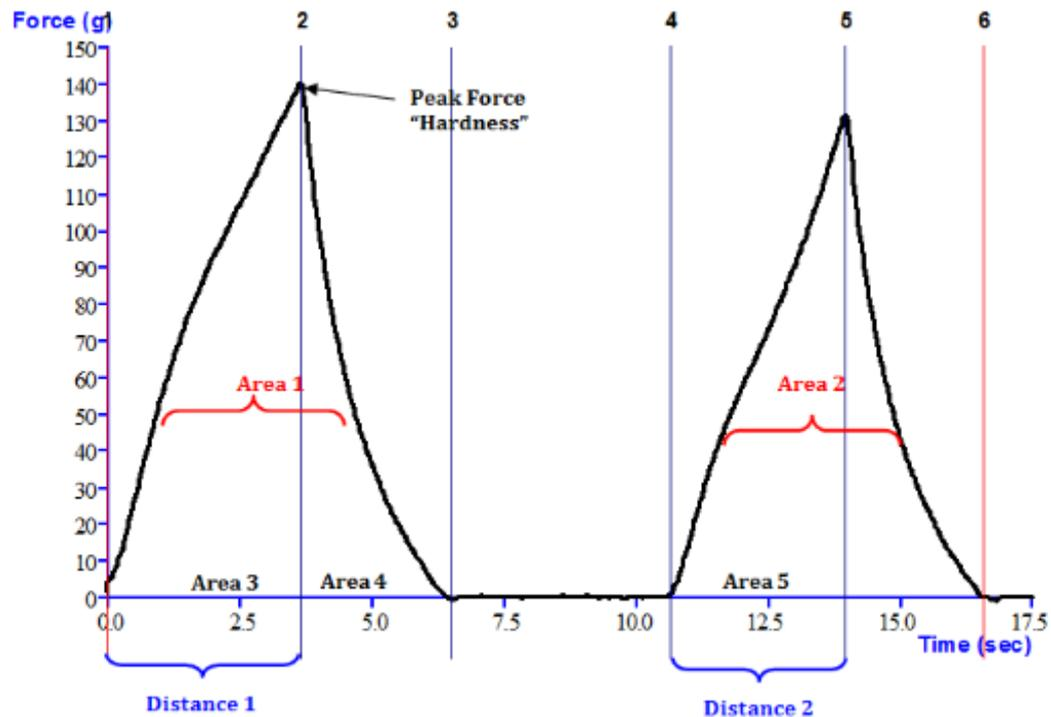
Figure 7 A plot of texture profile analysis calculation for texture expert software.
