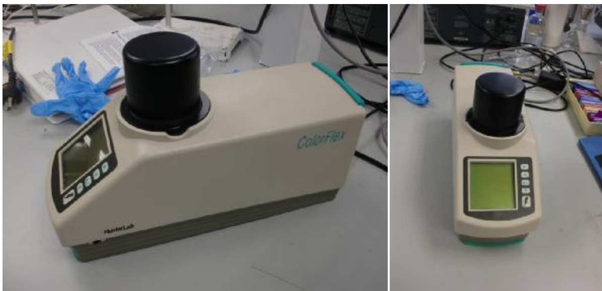
Figure 3.3 The Hunter meter with a shroud covering the crystallising dish that was placed centrally over the optical path
