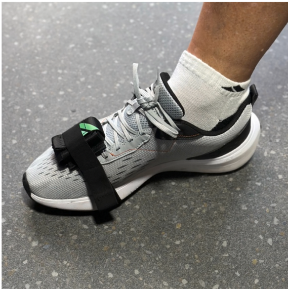
Fig. 7. Attachment of the IMU sensor to the shoe using a Velcro strap.
