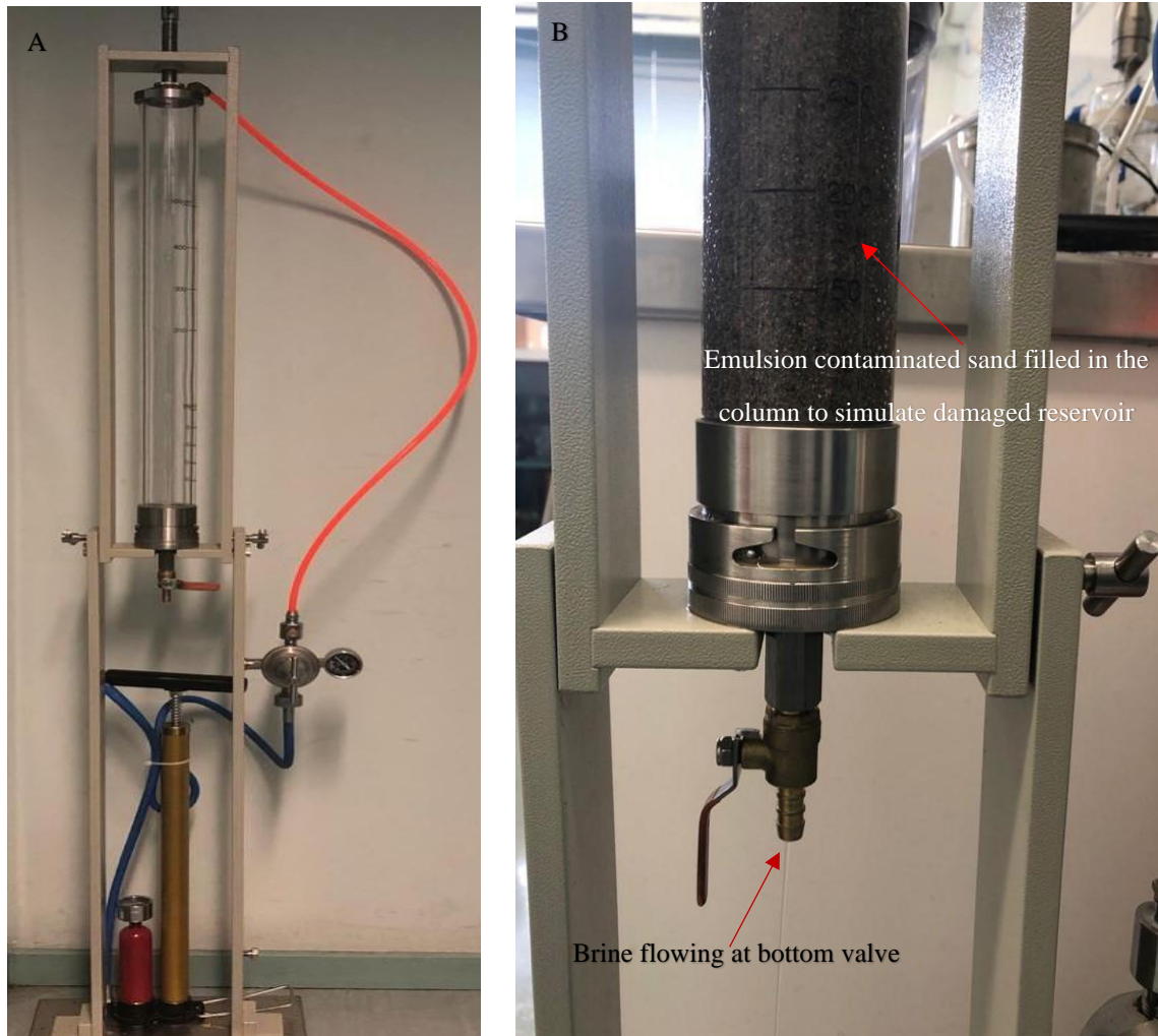
Figure 5.14: A) picture of empty sand packed column, B) picture of sand packed column filled with emulsion contaminated sand. Brine was filled and flowrate was determined for pre-treatment flowrate as a benchmark.
