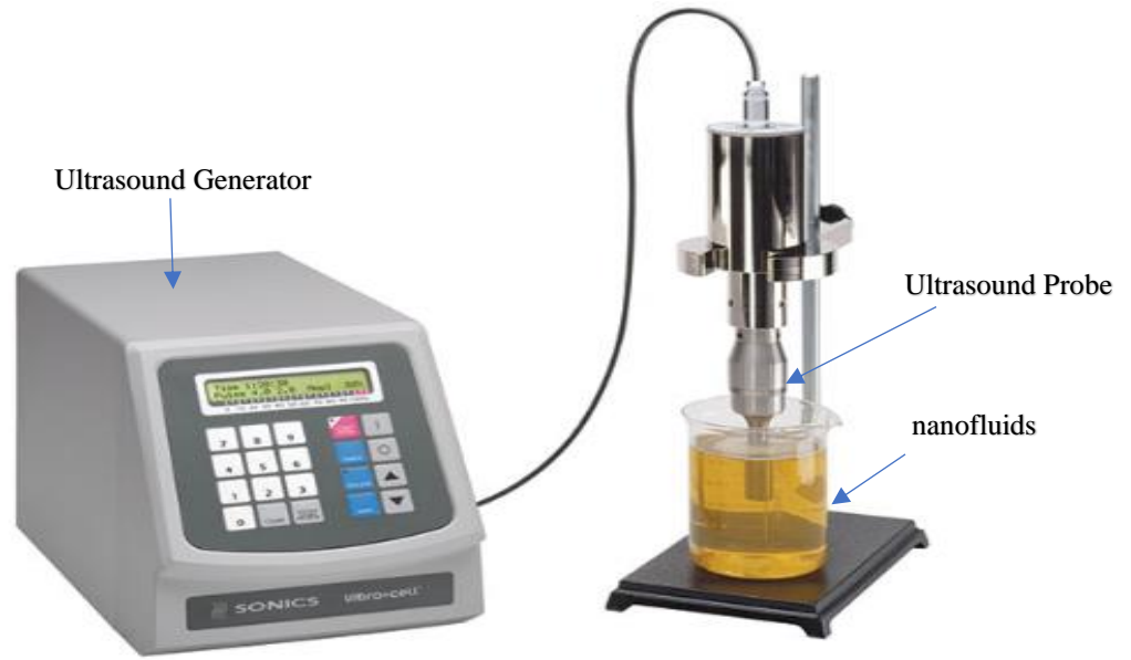
Figure 3.2: Picture of Nanofluids Preparation in laboratory (Image taken from SONICS & MATERIALS; INC ultrasonic VCX-500 liquid processor manual)
