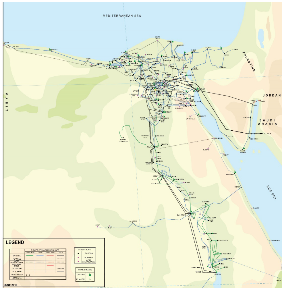
Figure (16): Egypt's national electrical grid [50].
