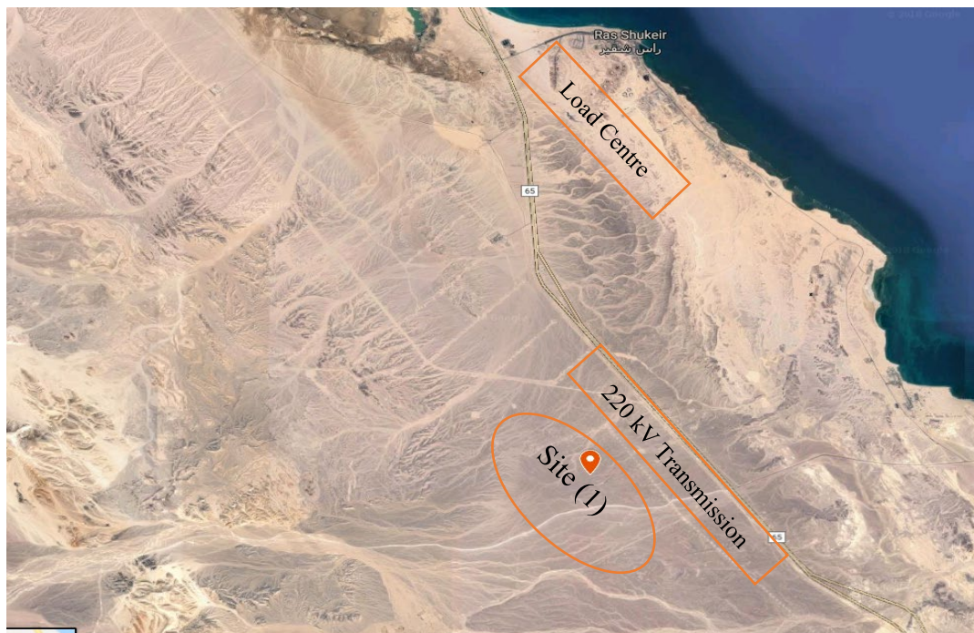
Figure (25): Map of the first selected site showing the transmission lines and load centre.
