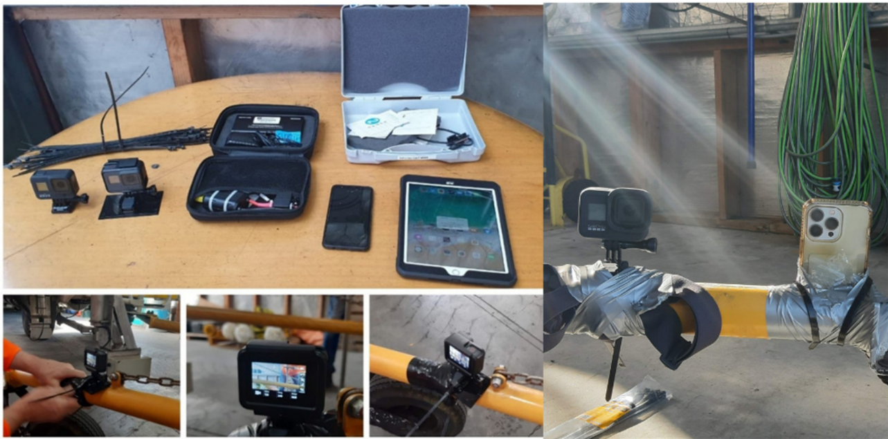
Figure 4. Data collection setup: iPhone 13 Pro (for LiDAR), Samsung A7 Mobile, Apple iPad 6, External power bank, GoPro cameras and mounting equipment, and camera and iPhone mounting on a BTM.
