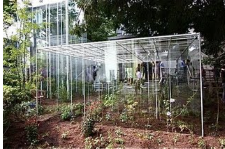
Fig. 27 "Extreme Nature" Project, glass structures sitting around landscape, 8mm thick glass and 16mm steel structure blend the inside and outside, image can be found at www.contessanally.blogspot.com
