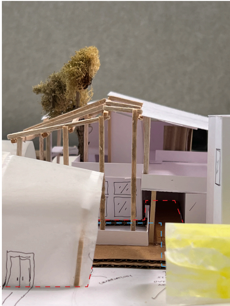
Figure 69. Working Model Frame 3. The fluctuation of vertical roof heights is illustrated. The open/enclosed pitched roof creates a double height volume on the ground floor and a single height volume in the veranda and communal rooftop, creating a sense of intimacy and shelter. The curve of the tunnel house is hinted at here, as well as its tangency to the main building, suggesting a loose L-shape form.
