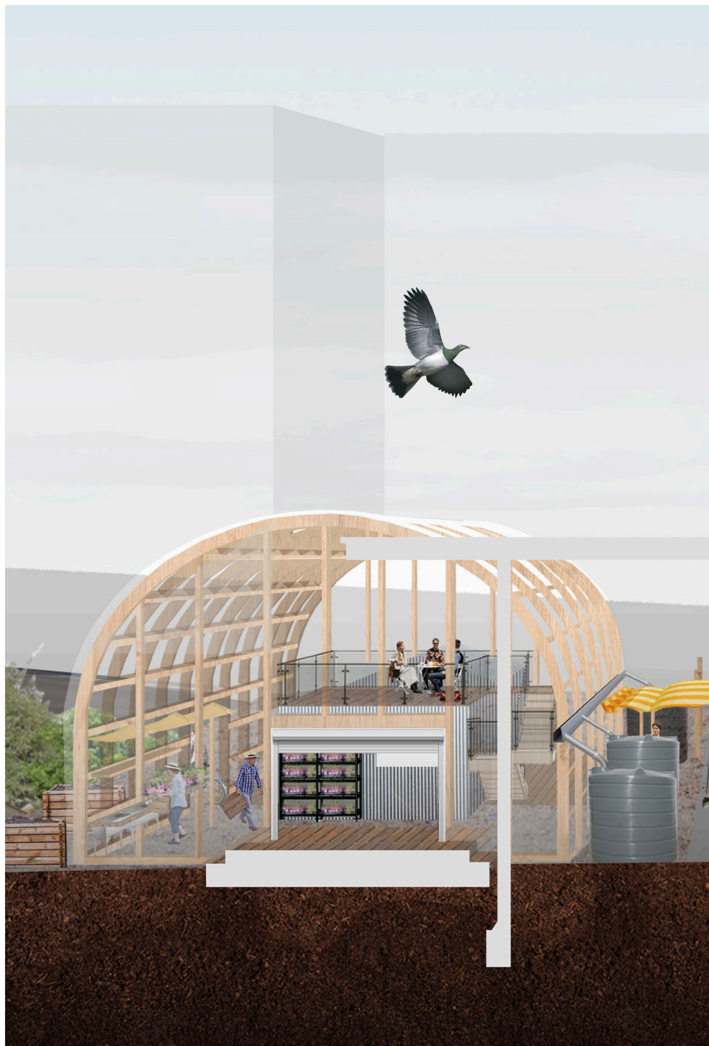
Figure 1. Tunnel House in Section.
