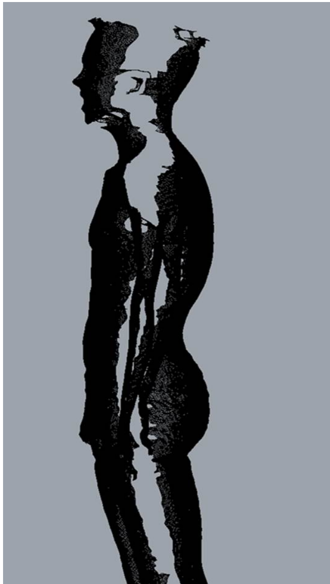
Figure 3. Extracted 3D body scan showing holes or dead angles within surface mesh.
