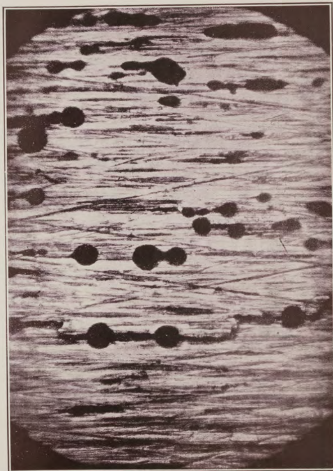
Fig. 1.—Corrosion fatigue fracture under jet of wet steam, of specimen 0.5 per cent. carbon steel X115. —From the "Journal of the Institute of Metals."
