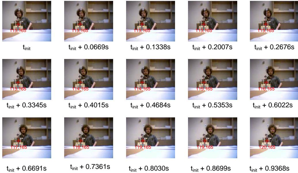
Fig. 6.13: This series of frames shows the reaction time of the CuWITH. Each frame has a cross (and a set of x,y coordinates) marking the location of the CuWITH. At  $t_{init}$  the person begins to move to the CuWITH's right, 401.5ms after the person starts to move CuWITH detects the movement and begins to follow the person to the right
