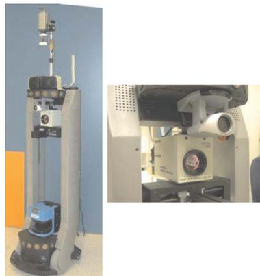
Fig. 2.2: The ActivMedia Peoplebot robot used as the experimental platform by Treptow et al. (2005).
