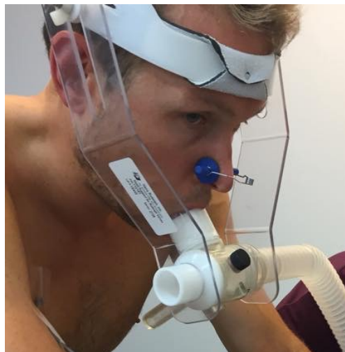
Figure 2. Expired gas collection during cycling exercise
